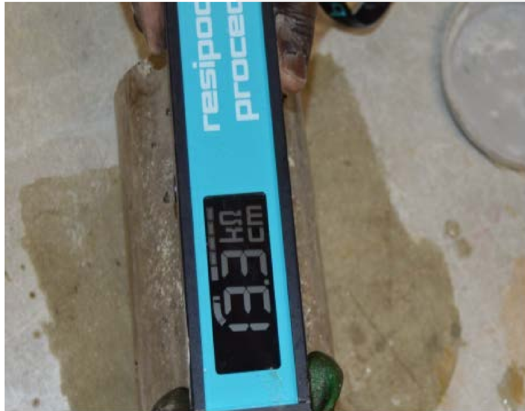
Figure 1- Surface resistivity testing.
