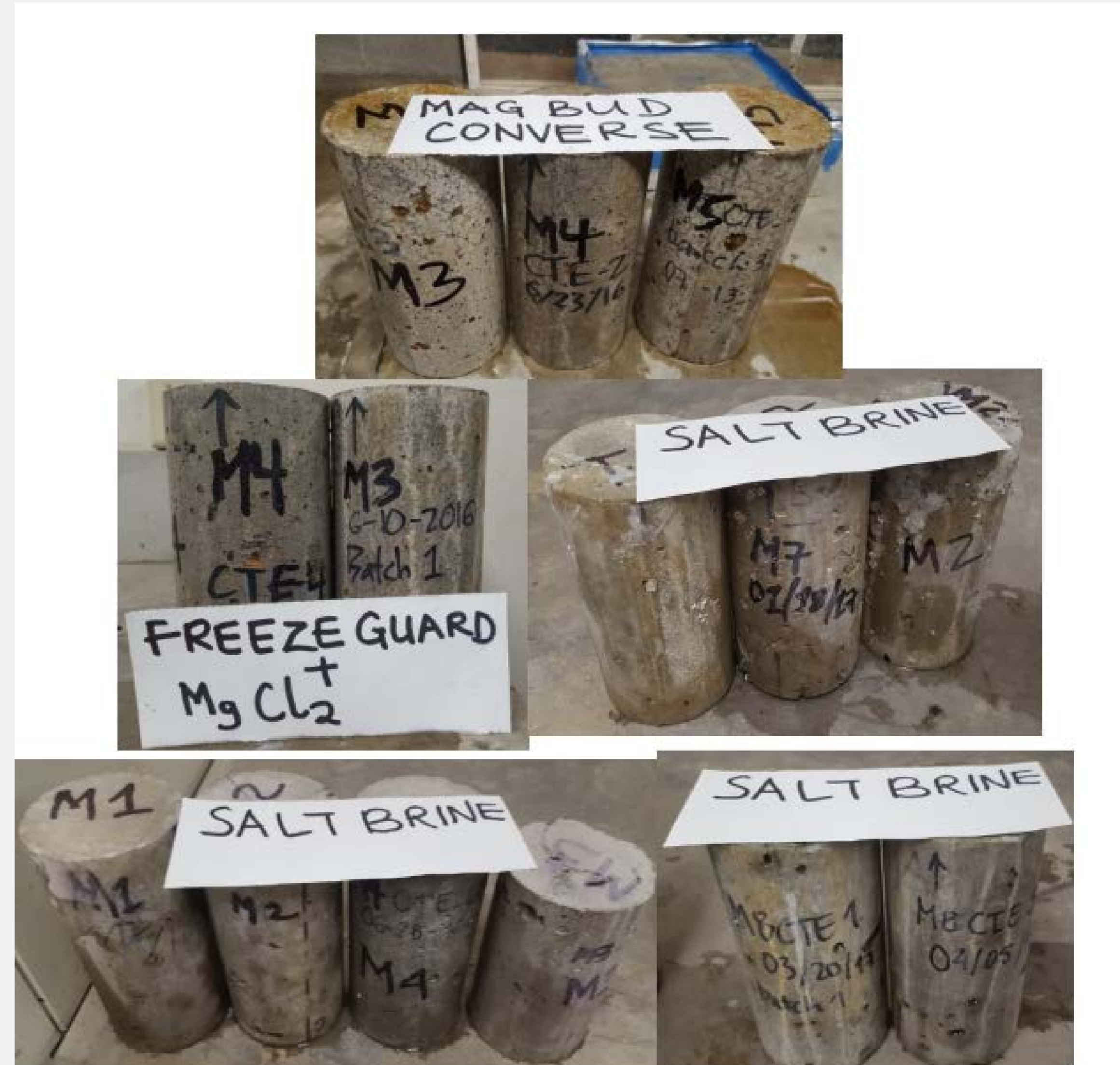
Figure 15: Concrete specimens after 90-days continuous soaking in deicing salt.
