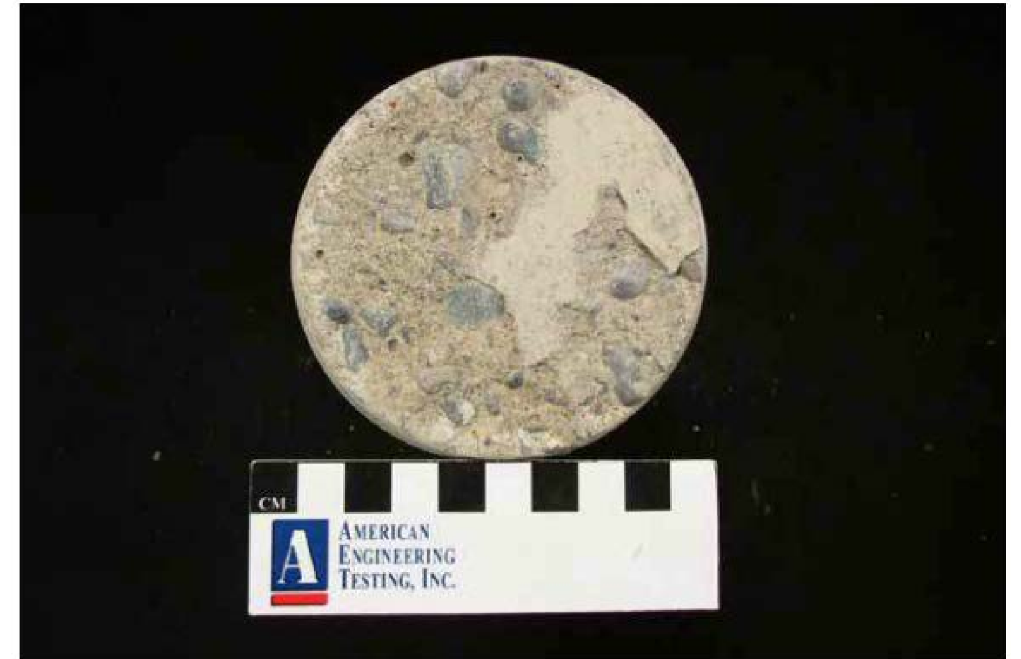
S-10 DESCRIPTION: Mostly scaled front surface of the core sample as received.
