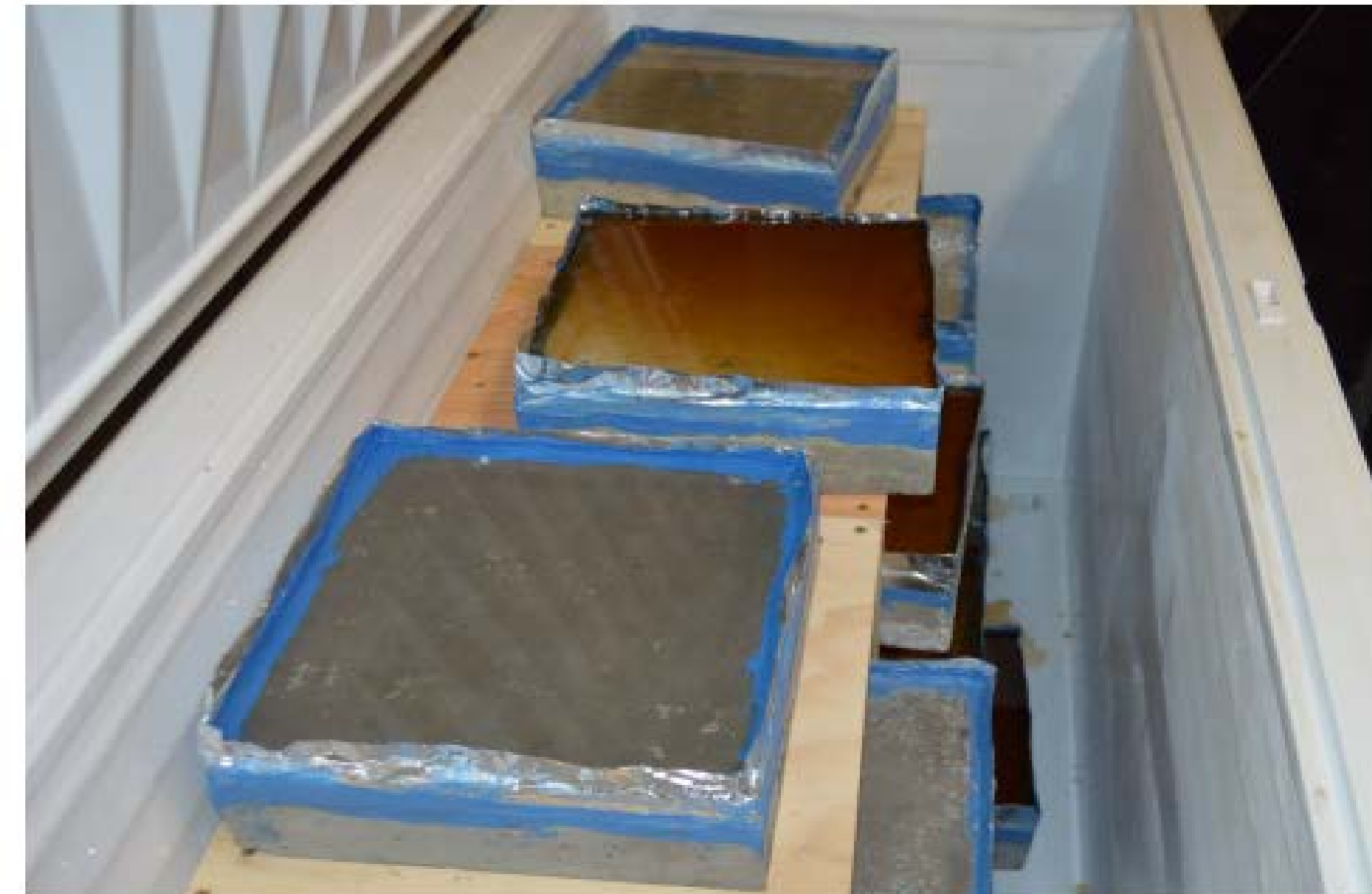
Figure 3: Slabs exposed to freezing environment during deicing scaling test.
