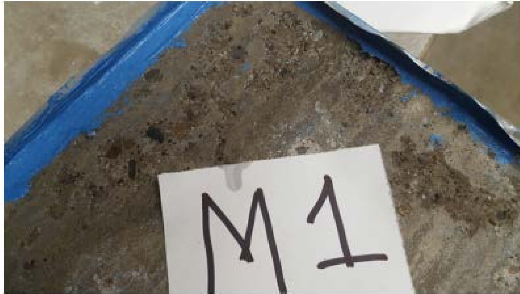
Figure 7: District 1 SH 5 Crossing mixture after deicing scaling test
