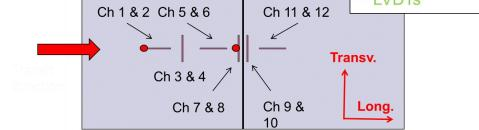
Gages oriented in the longitudinal axis and placed at the bottom and closed the joint will be studied. These are Ch. 6 and 12.
