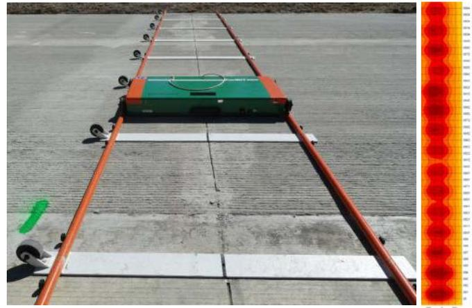
The major benefits of MIT Scan 2 are that it is nondestructive, measurement can be taken extremely quickly (two to five minutes per joint), results can be seen in a graphical display or a tabular format immediately in the field for quality control purposes, and it is not very complicated to operate. Currently North Carolina DOT, Nevada DOT, and the New York Thruway Authority, have specified the use of this technology to check alignment of dowel bars in their specifications.
