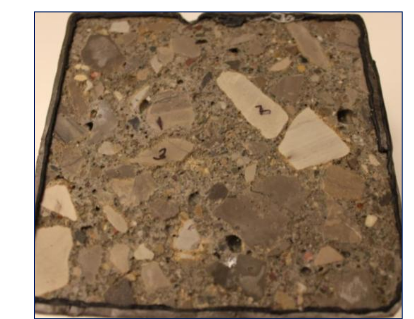
Silane treated specimen
