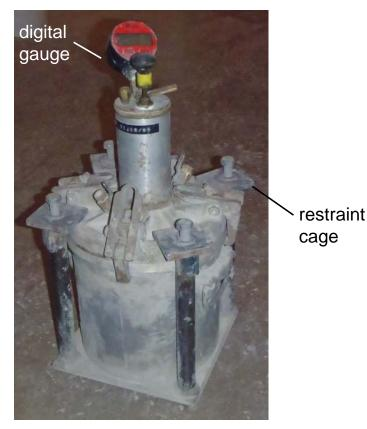
The current version of the meter uses a digital pressure gage and a restraint cage. The next generation of the meter will not require a restrain cage and provides a digital gage that provides the user with the total volume of air and the spacing factor. The gage will also be able to tell the user if they have run the test correctly.
