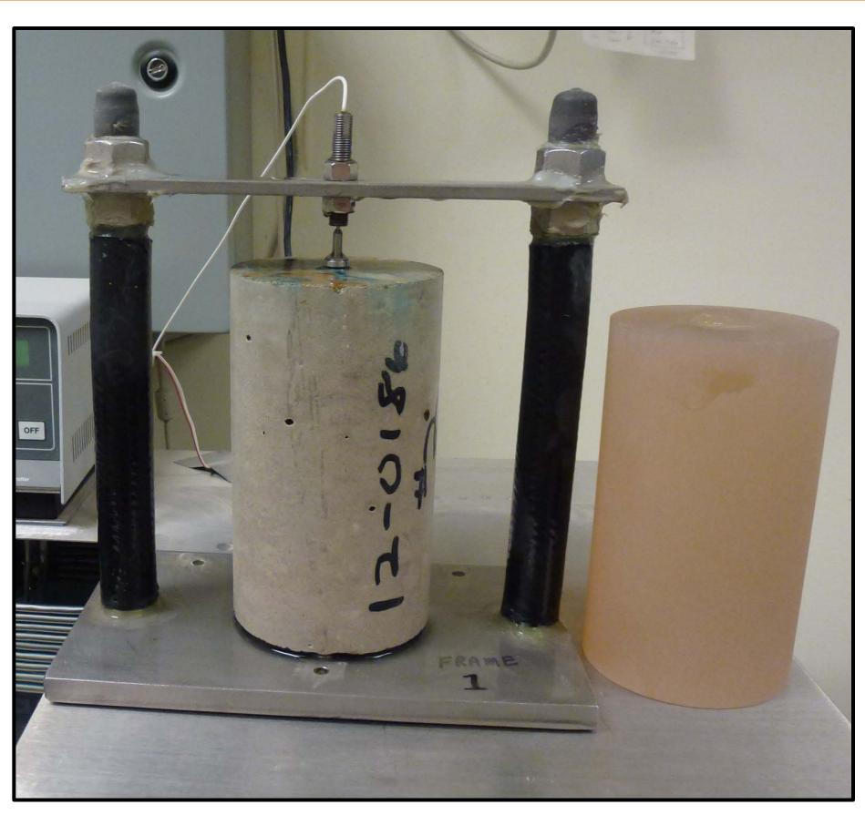
Figure 2: CoTE Test Frame with Sample and Ceramic Cylinder
