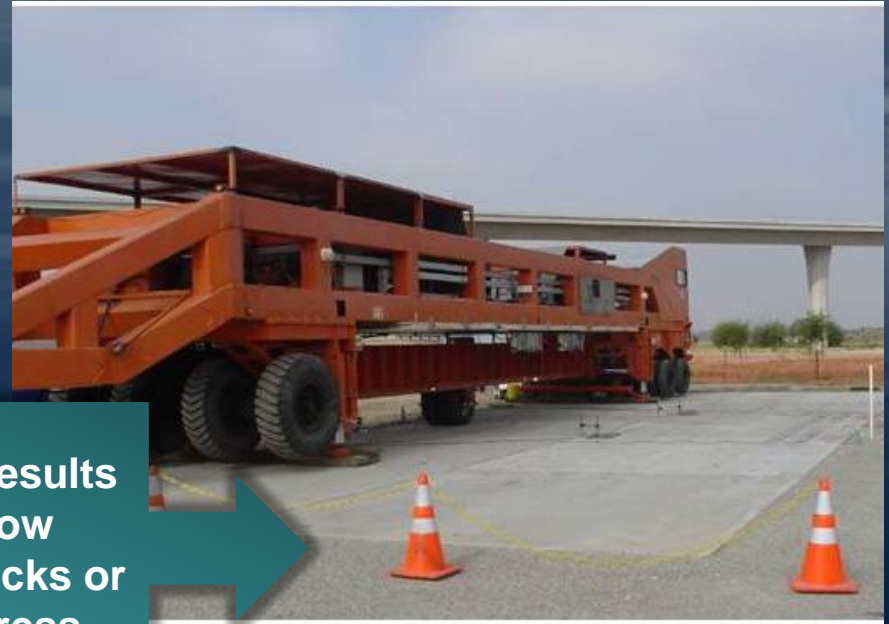
Heavy vehicle simulator 143 Million ESALs (100 KN Load) 4.3 Million Cycles
