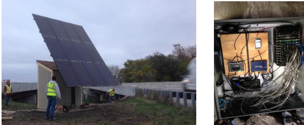
Figure 8. Similar field site with field equipment and solar power for typical SHM system on the I-280 EB Bridge in Illinois over US 67 near Milan
