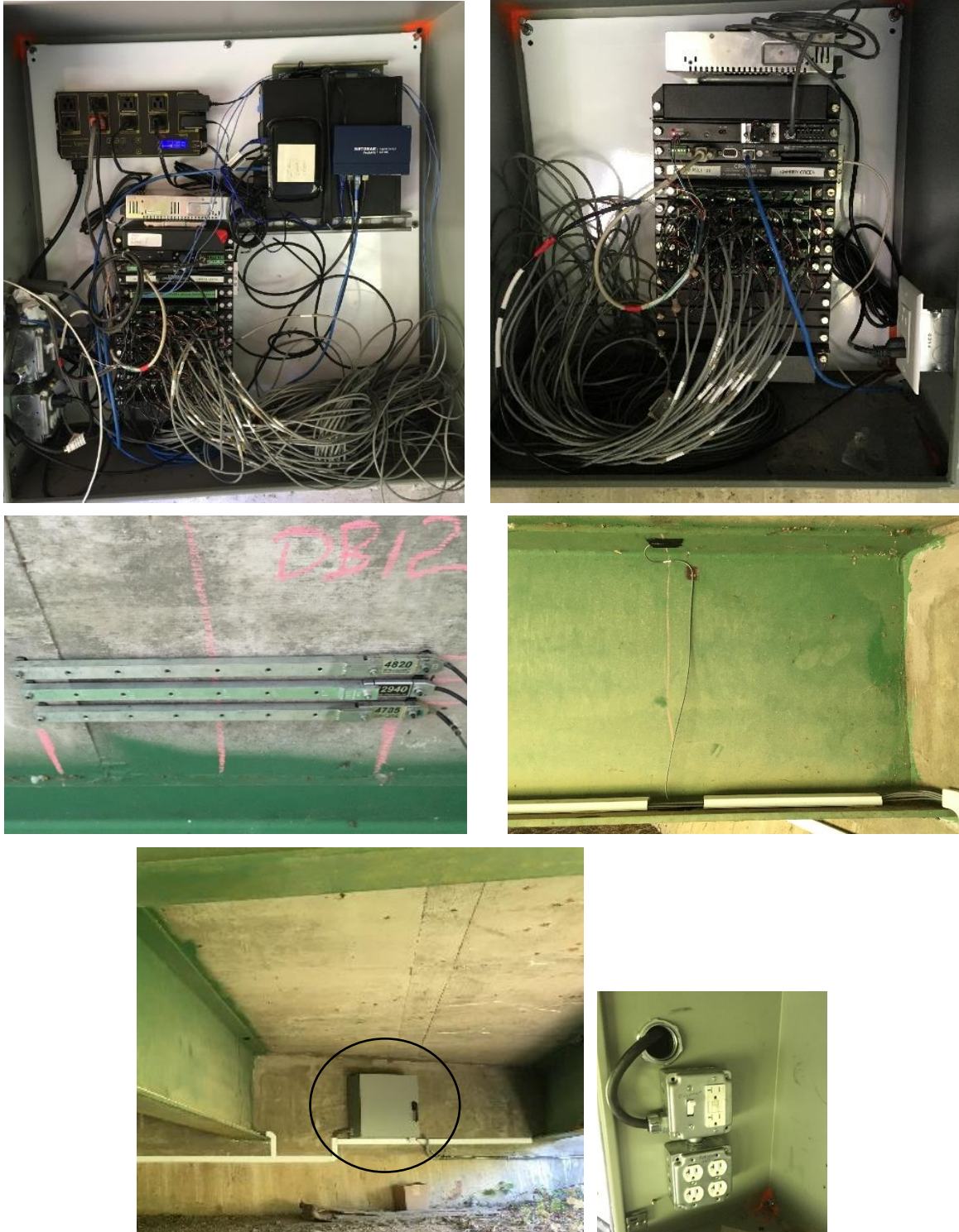
Figure 14. Field hardware and components: typical hardware for the SHM system (top), bridge deck strain gauges (center left), steel girder strain gauges (center right), and cabinet containing data and communication under the bridge site with power provided at the site (bottom)
