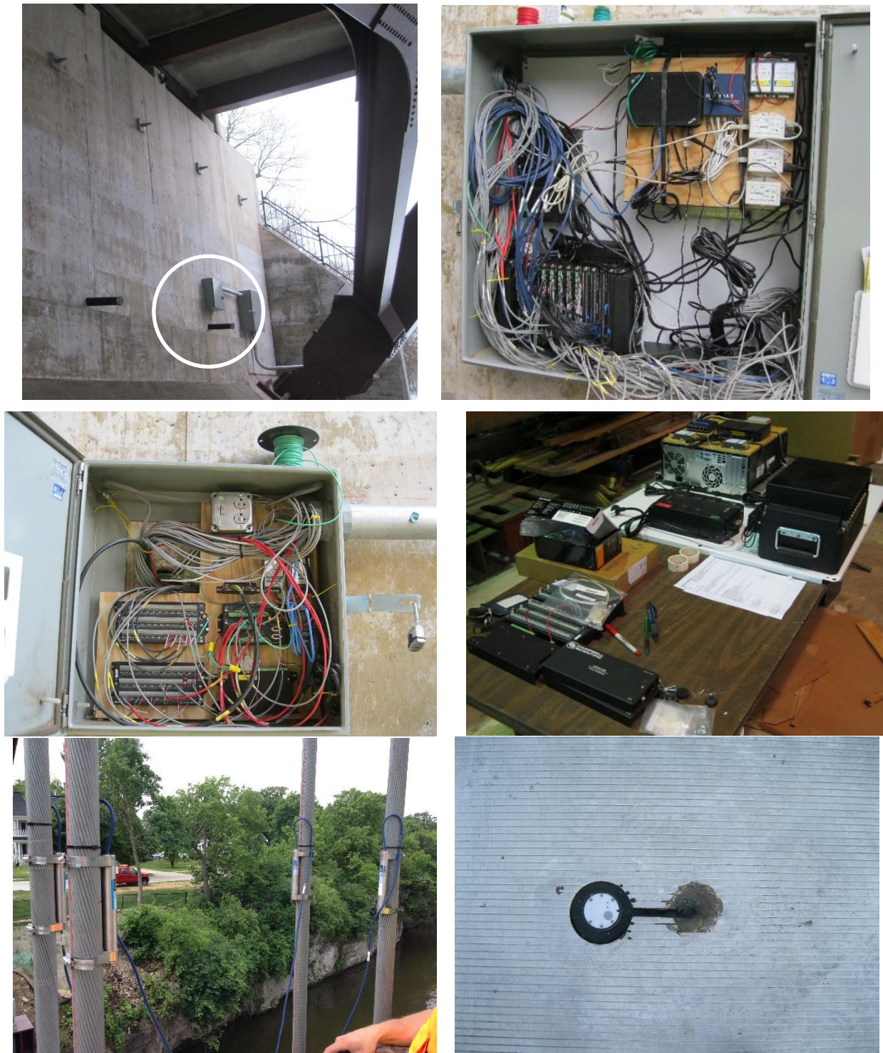
Figure 18. SHM system components associated with the US 65 Bridge over the Iowa River: data collected at the bridge site (top left), data logging equipment (top right), additional hardware (middle left), organizing home base to connect to ISU (middle right), strain gauges on hangers (bottom left), and bridge deck sensor placed in the deck (bottom right)
