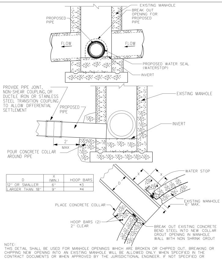
ALLOWED, A CORED OPENING SHALL BE REQUIRED. FOR CORED OPENINGS, INSTALL A FLEXIBLE WATER TIGHT CONNECTION PER 6020, 2.01I. DO NOT GROUT CORED OPENING.
