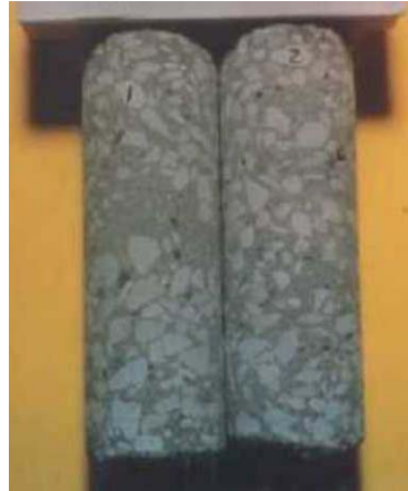
Left core - aggregate segregation
