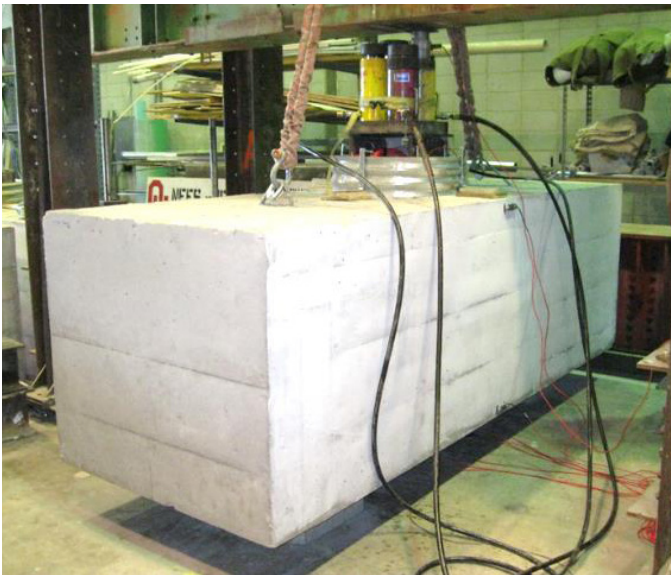
Pile-to-pile cap connection specimen in reaction frame for load testing
