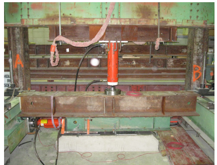
Coefficient of friction test setup, showing stainless steel sole plate and PTFE-topped neoprene bearing pads
