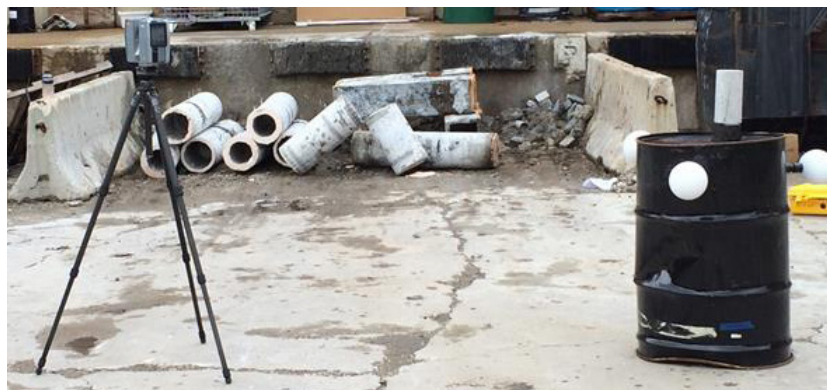
Laser scanning a concrete cylinder
