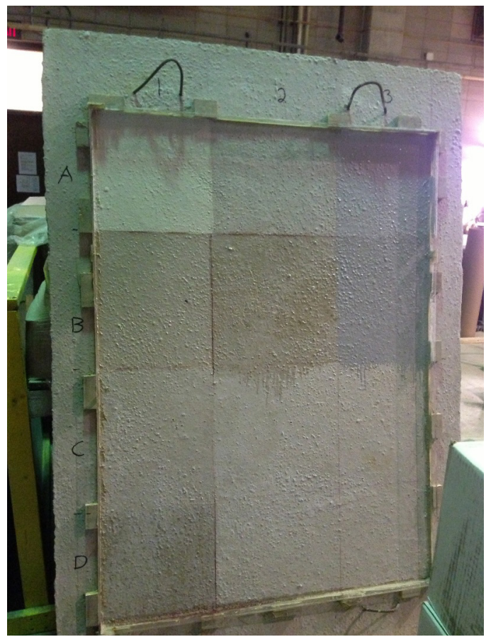
Typical ponding slab with coating alternatives applied
