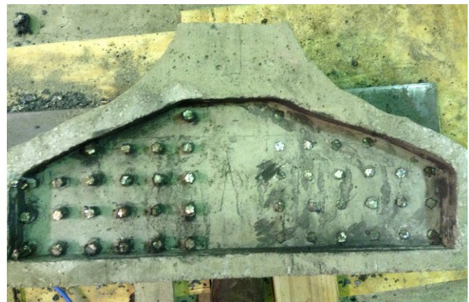
Single blockout formed with 2 in. foam
