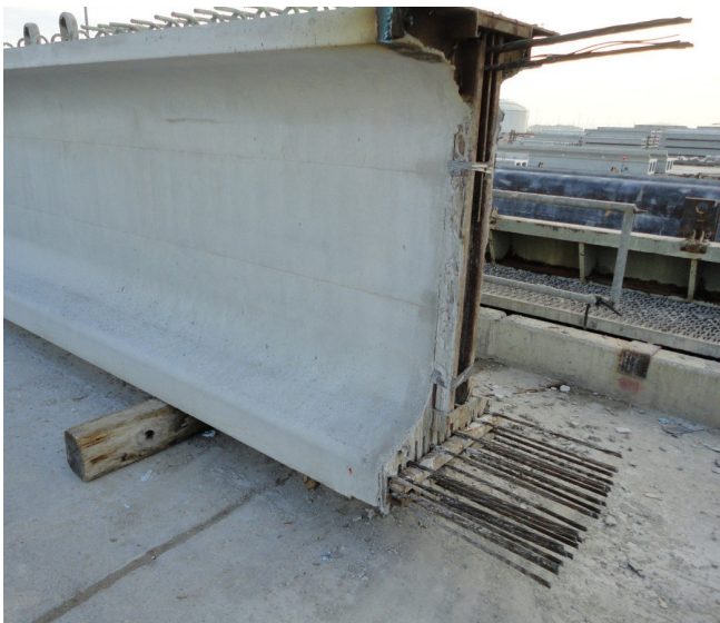
Overhang distances of the PPCB ends vary during storage on temporary supports at the precast plants
