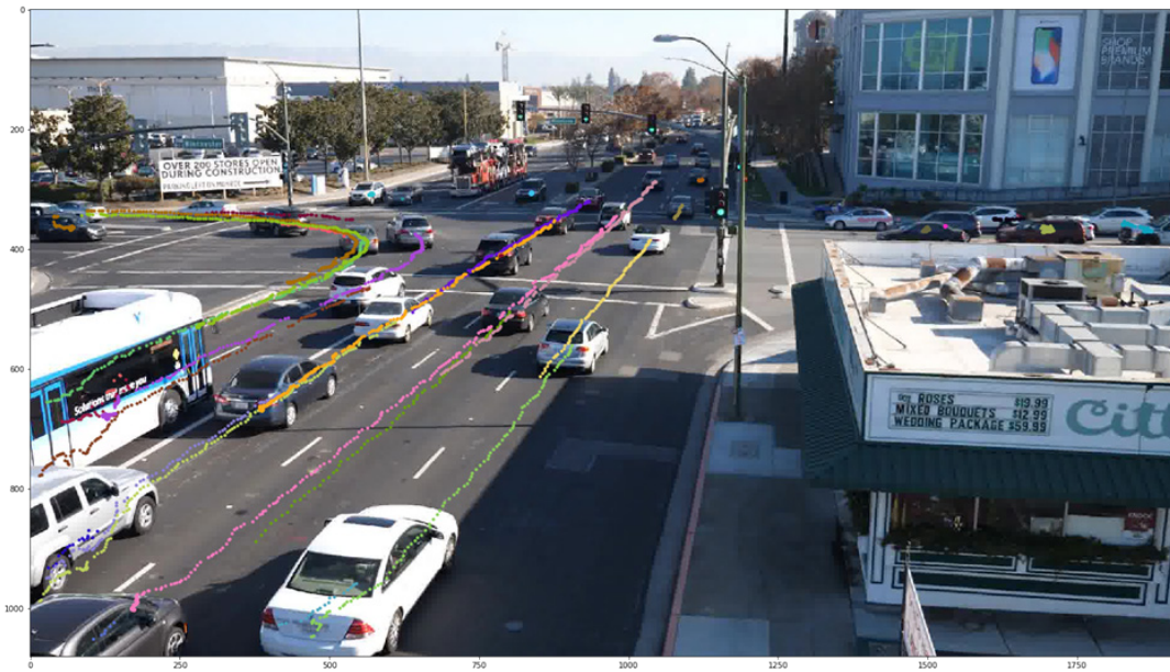
Sample vehicle detection results obtained from videos recorded at Stevens Creek and Winchester intersection in Santa Clara, California
