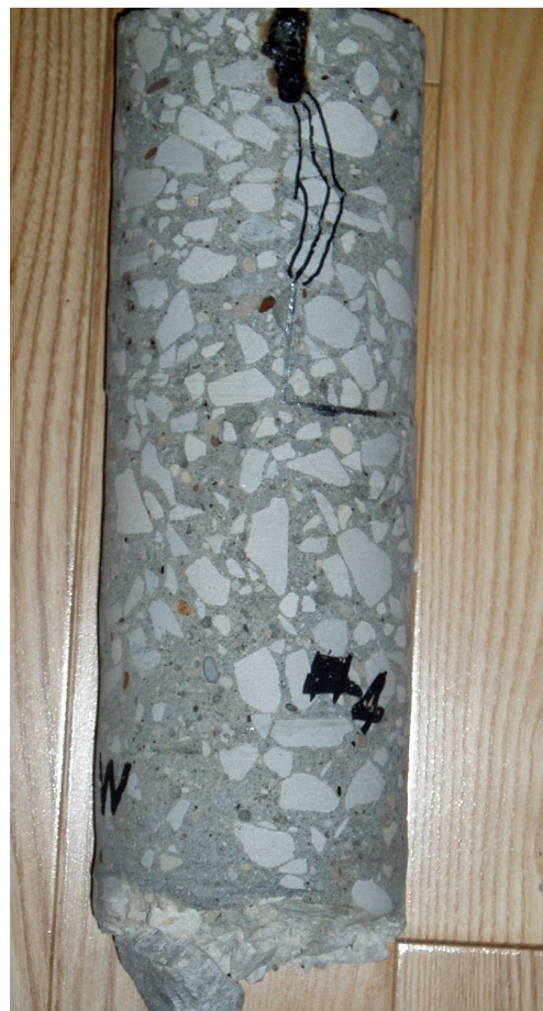
Core sample showing a crack extending from the joint former
