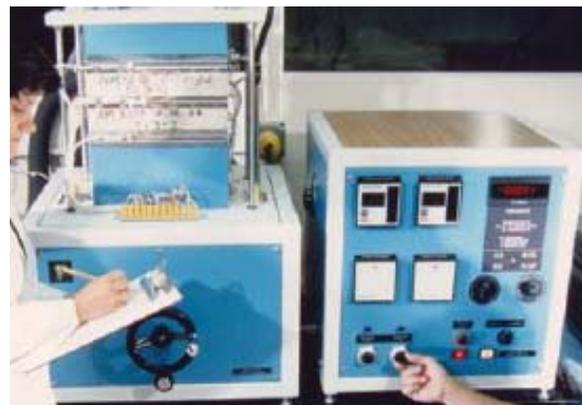
*Test setup for thermal conductivity*
