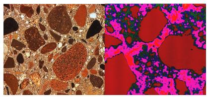
Concrete slice (left) and false color concrete image (right)
