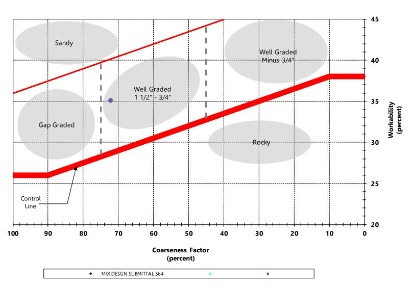
Figure 6. SR-46 Combined Gradation Coarseness and Workability Factors
