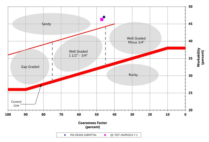
Figure 6. I-80 Combined Gradation Coarseness and Workability Factors
