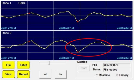
*Figure 8. GSI Screen Showing a Dip and Bump (red oval) Where the Stringless System Malfunctioned*
