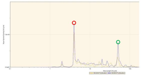
Figure 7. Power Spectral Density Analysis from August 11 and 13, 2015 for Trace 2 (right wheel path of the driving lane)
