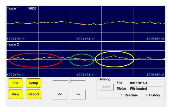
Figure 9. GSI Screen Showing Event Markers for Rough and Unstable Paver Trackline (red oval), Paver Stop (green oval) and Overloaded Paver (yellow oval).
