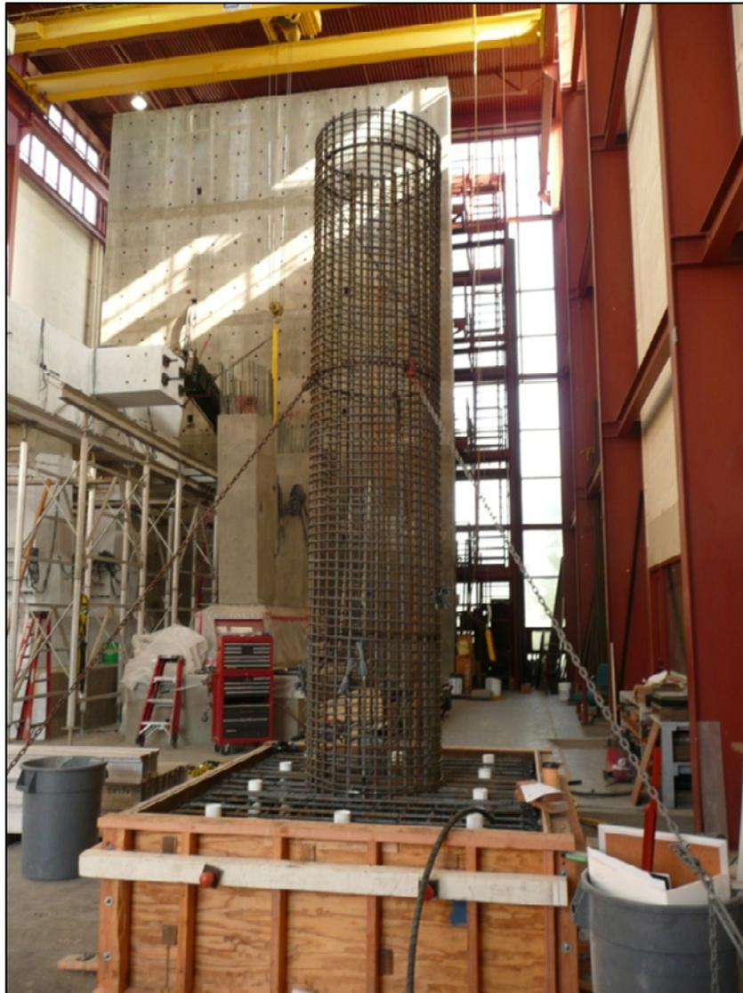
Figure 5.2: Completed Column and Footing Cage
