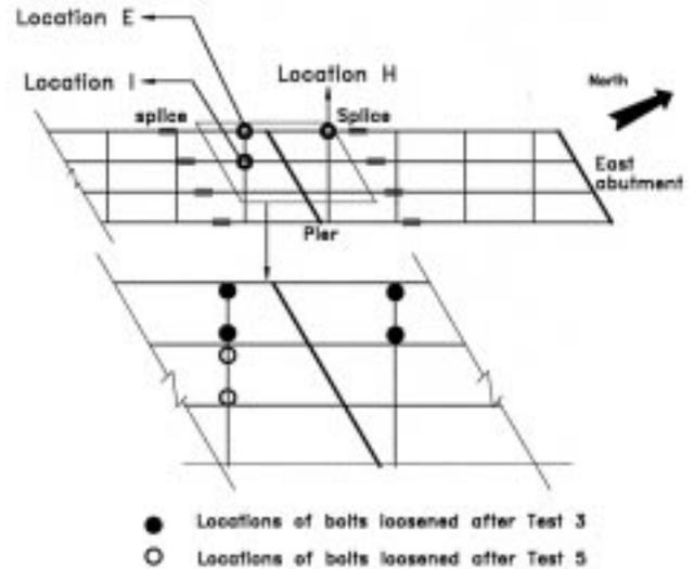
FIGURE 3 Schematic plan showing the instrumentation locations.
