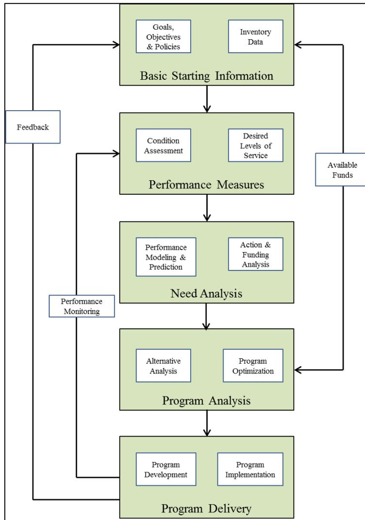
**Figure 2.1. Components of an asset management system (Smith 2005)**
