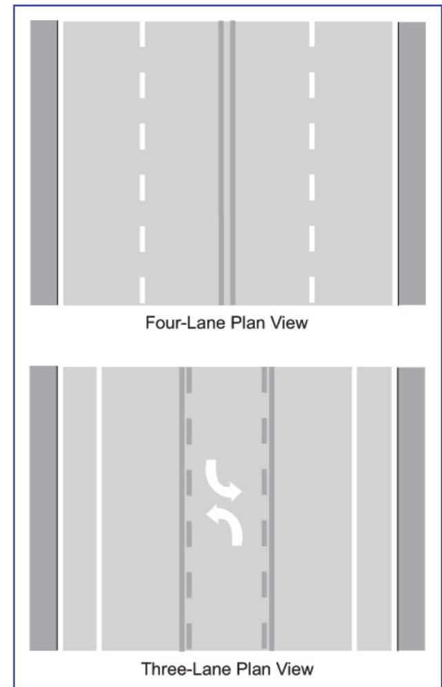
**The use of non-traversable medians helps delineate travel lanes, separating left turns from through traffic.**
