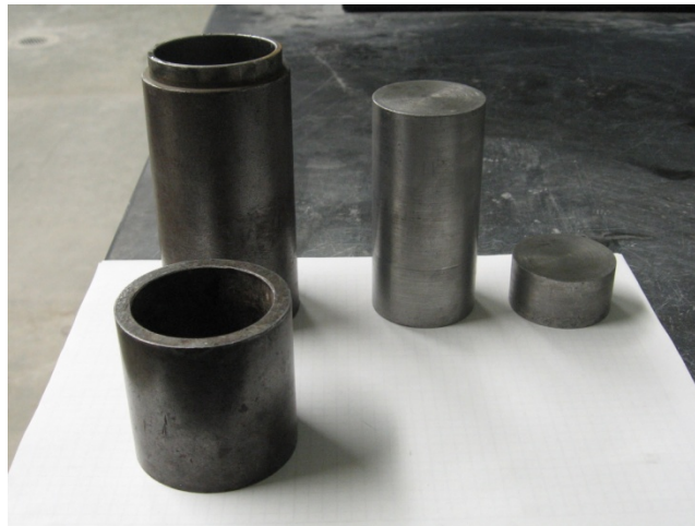
Figure 9. Mold apparatuses for static compaction
