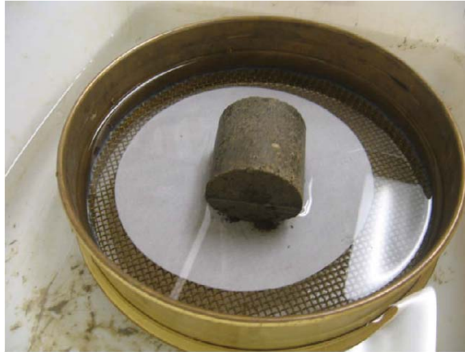
Figure 19. Example of fly ash treated specimen under half-saturation procedure
