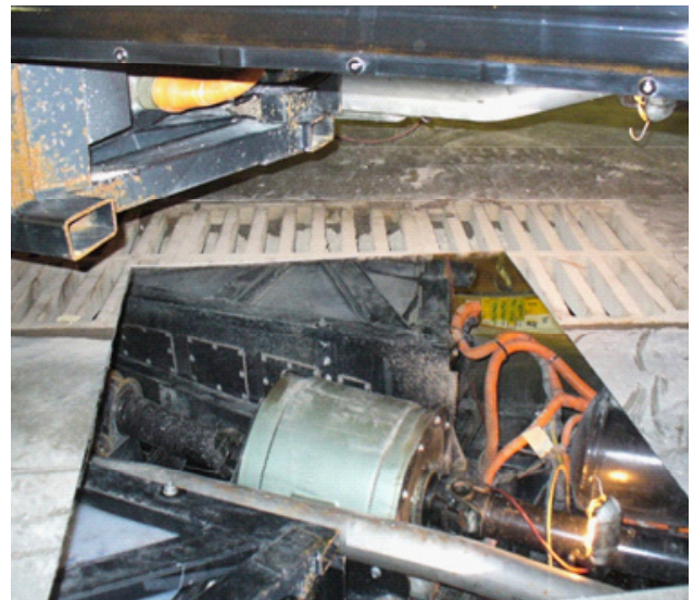
Hybrid-electric power train, shown in mirror on floor
