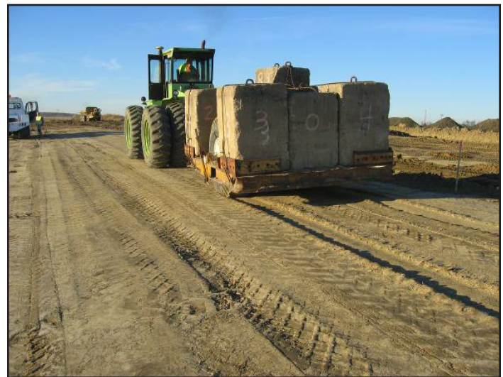
Figure 7. Test roller and subgrade rutting observed following test rolling (from Thompson et al. 2008)
