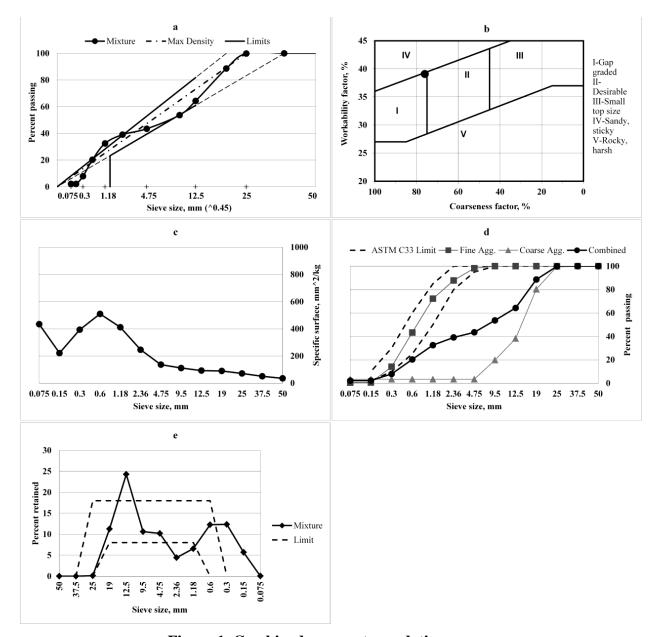
Figure 1. Combined aggregate gradation curves
