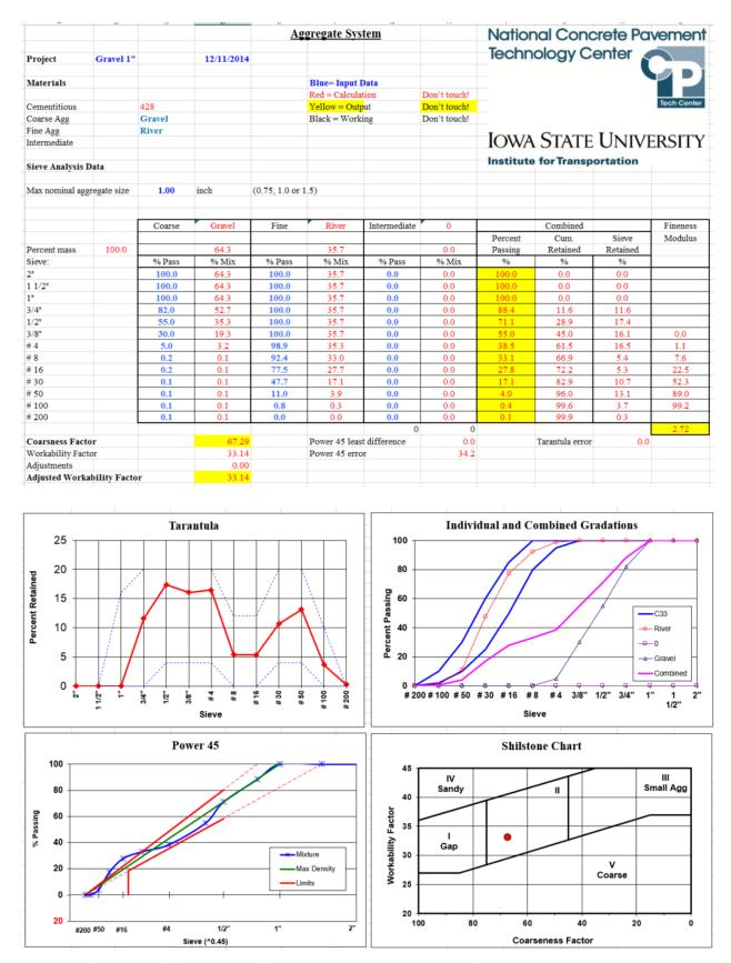
Figure 13. Screenshots from the spreadsheet pages for the aggregate system
