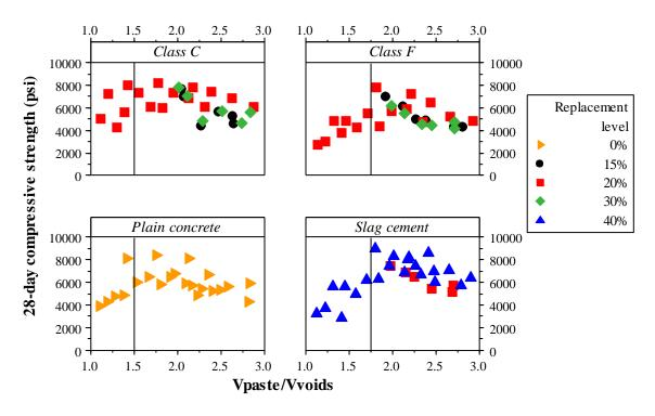
Figure 7. Required paste system for 28-day compressive strength
