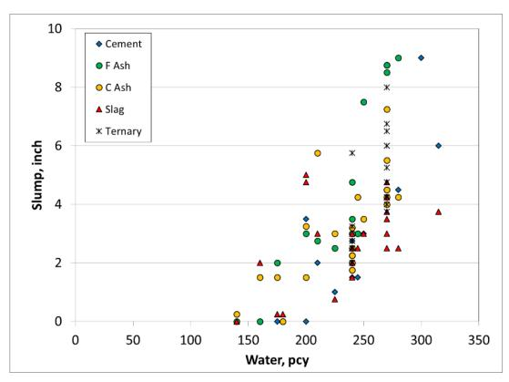
Figure 2. Effect of water content on workability
