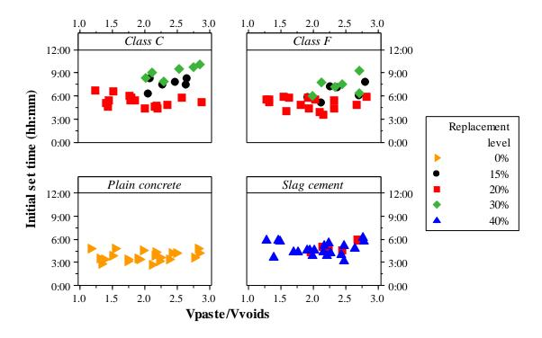
Figure 5. Required paste system for initial set time
