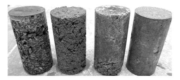
Figure 4. Cylinders made with mixtures with increasing cementitious content from 400 to 700 lb./yd.<sup>3</sup>
