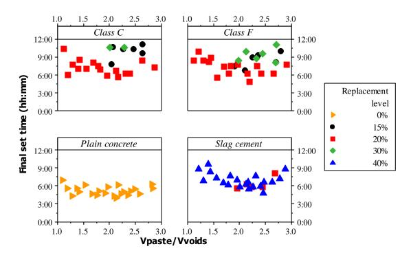
Figure 6. Required paste system for final set time
