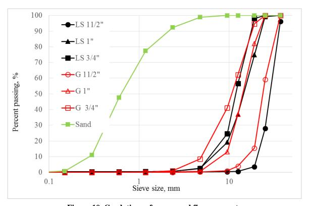
Figure 10. Gradations of coarse and fine aggregate
