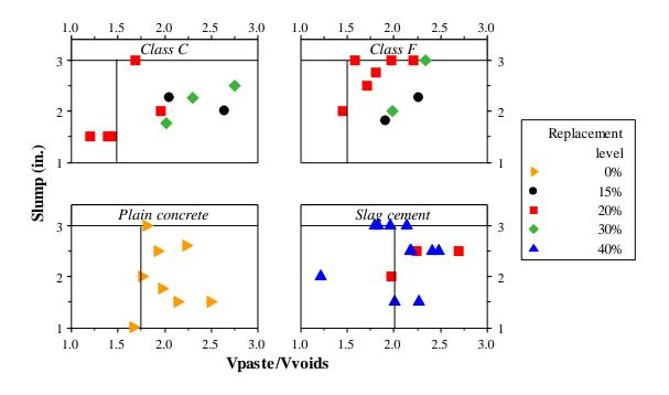
Figure 3. Required paste system for workability
