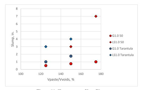
Figure 11. Slump versus  $V_{paste}/V_{voids}$
