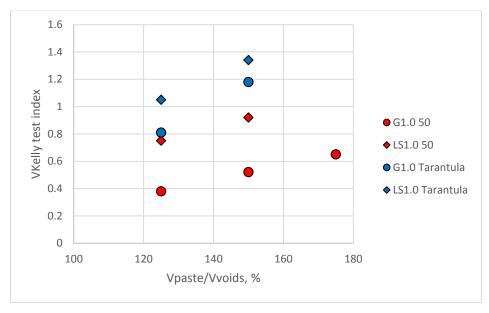
Figure 12. VKelly test index versus V<sub>paste</sub>/V<sub>voids</sub>
