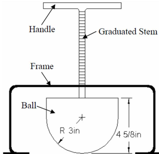
**Figure 1. Kelly ball test apparatus (Koehler and Fowler 2003)**
