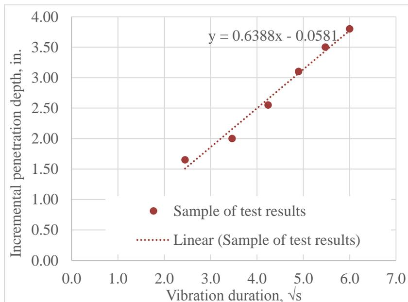
**Figure 7. Sample plot of VKelly test results**
