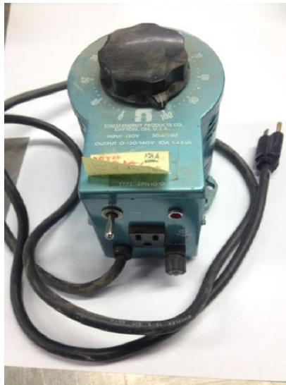
**Figure 4. Variable transformer**
