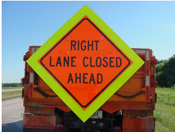
Figure 4. Orange RIGHT LANE CLOSED AHEAD Sign With FYG Background
