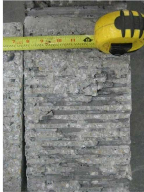
b) Failure interface of specimen with fluted surface and no interface reinforcement
