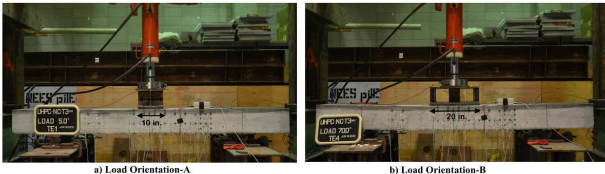
**Figure 26. Load orientations used in flexural testing of composite deck specimen**
