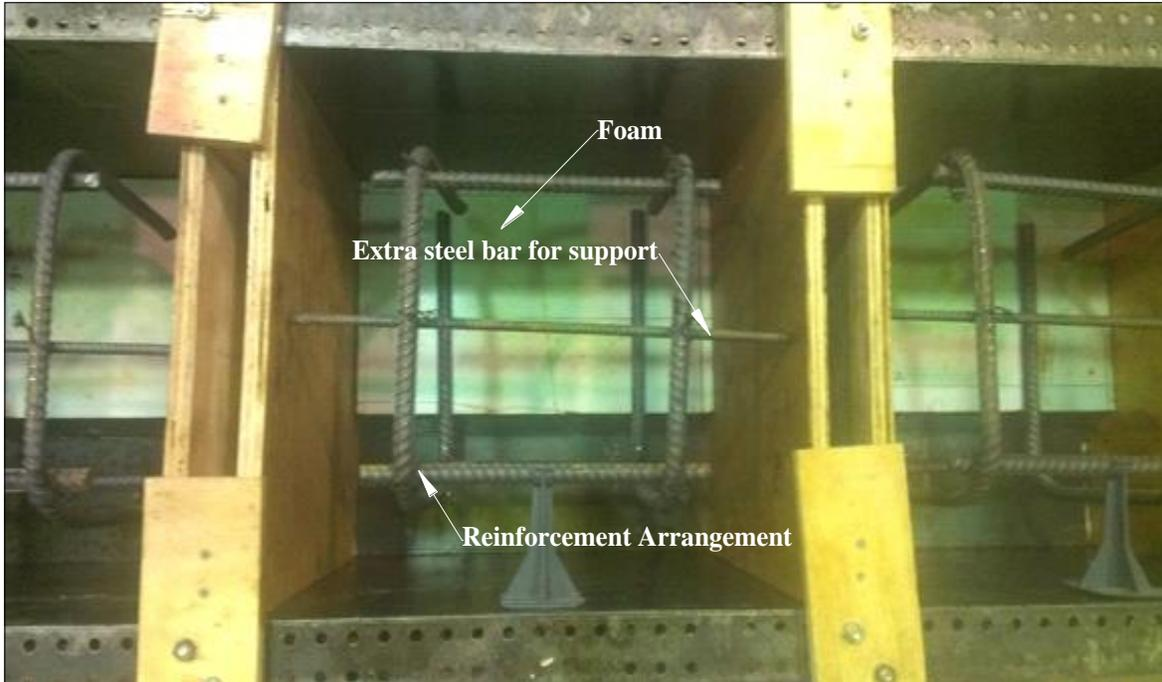
**Figure 27. Push-out test formwork for substrate concrete placement**
