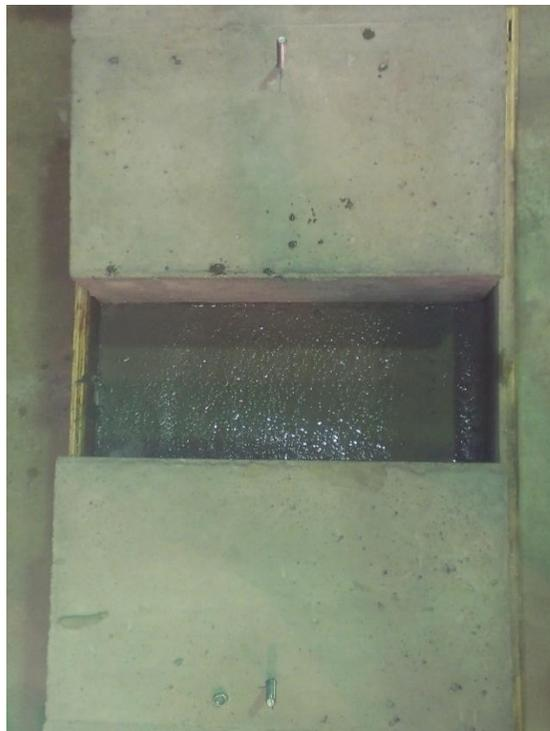
**Figure 31. Push-out test specimen after overlay concrete placement**
