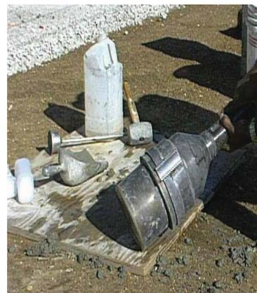
Devices for air content measurement of fresh concrete
