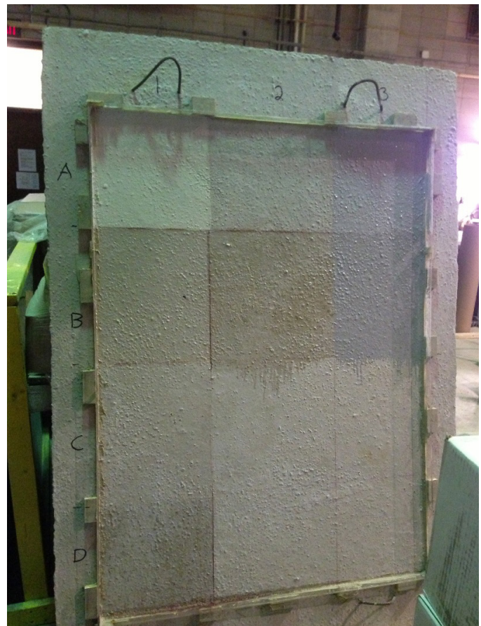
Typical ponding slab with coating alternatives applied
