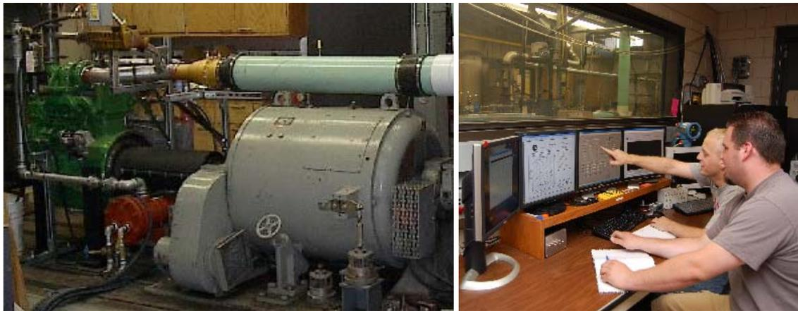
**Figure 4-1. Test engine, dynamometer, and the control room in the engine laboratory**
