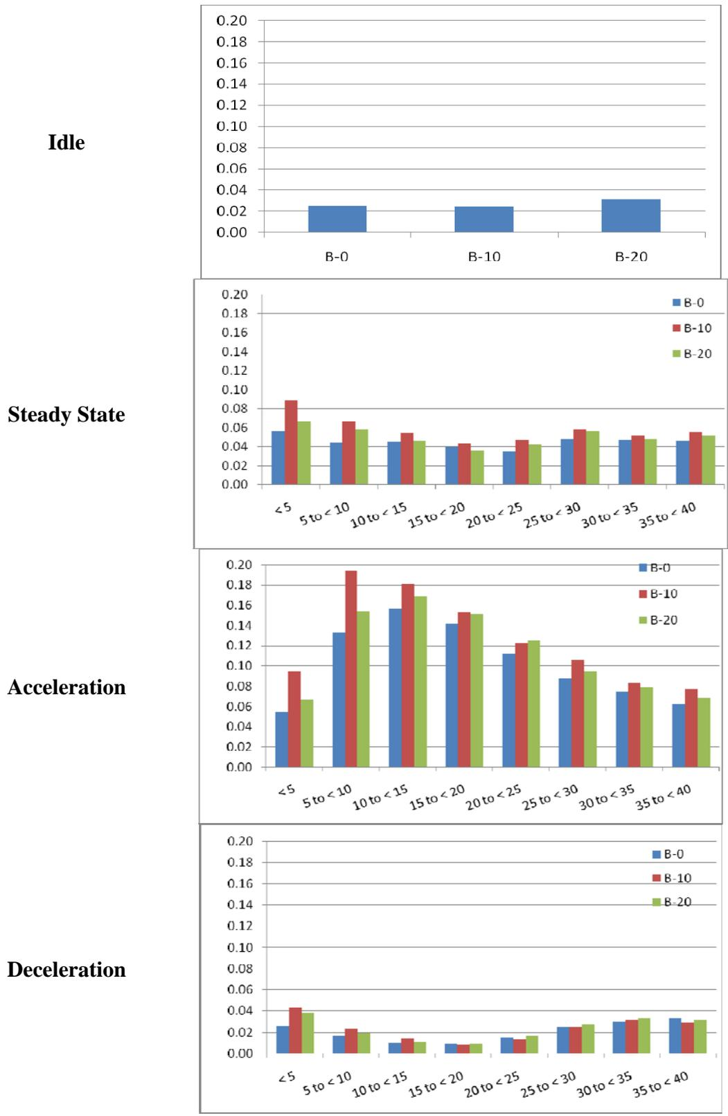
Figure 3-29. NO<sub>x</sub> emissions (g/s) for Bus 997 by mode and speed (mph)
