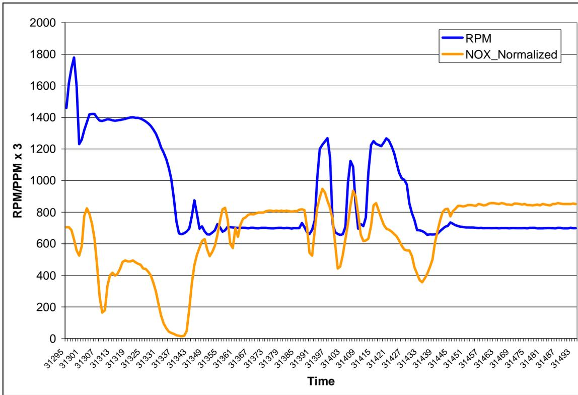
**Figure 3-6. Plot of RPM versus NO<sub>x</sub> to check for synchronization (NO<sub>x</sub> was multiplied by a factor of 3 for graphing purposes)**
