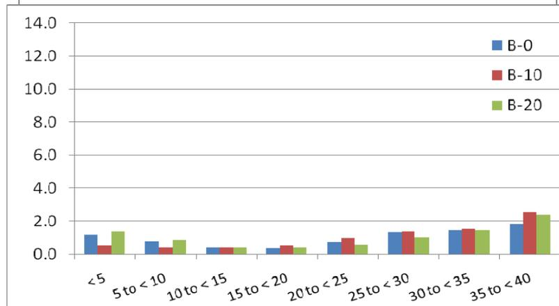
**Figure 3-26. CO<sub>2</sub> emissions (g/s) for Bus 971 by mode and speed (mph)**
