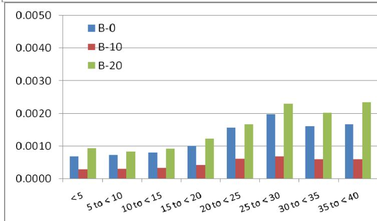
**Figure 3-22. HC emissions (g/s) for Bus 971 by mode and speed (mph)**
