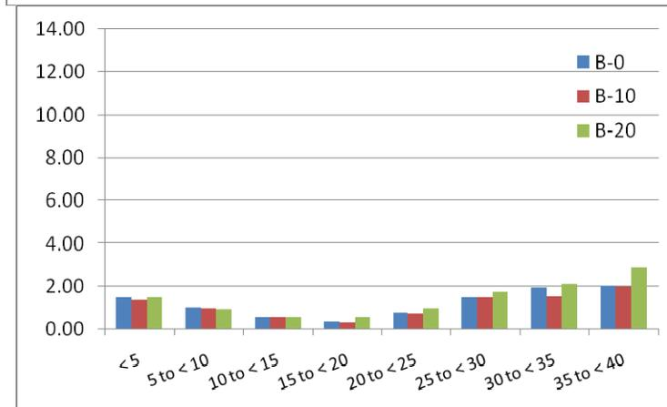
**Figure 3-16. CO<sub>2</sub> emissions (g/s) for Bus 973 by mode and speed (mph)**
