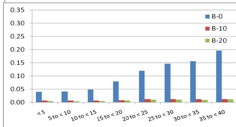
**Figure 3-27. PM emissions (mg/s) for Bus 971 by mode and speed (mph)**
