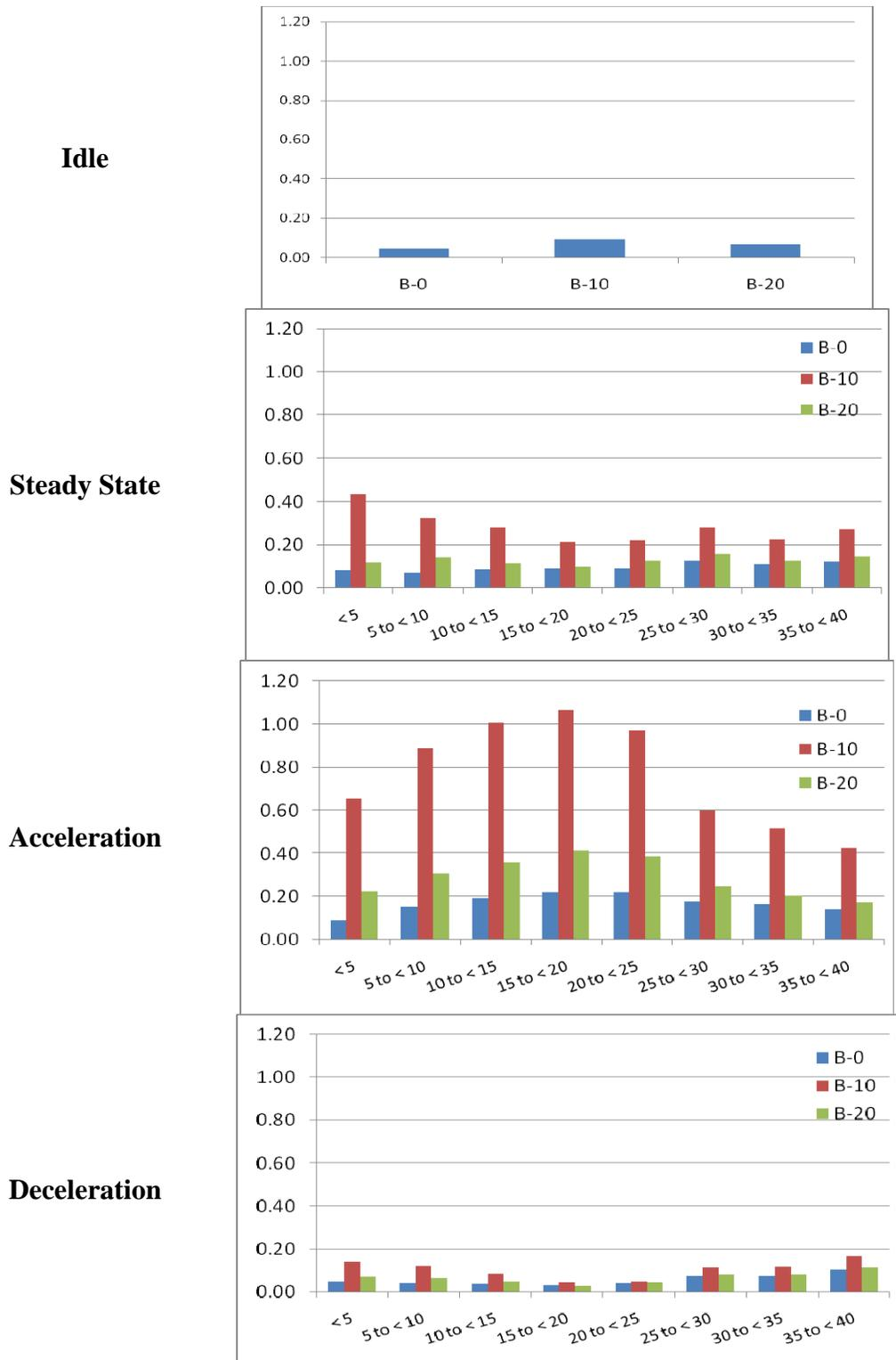
Figure 3-37. PM emissions (mg/s) for Bus 997 by mode and speed (mph)
