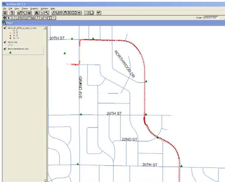
**Figure 3-5. HC for Bus 1-A along route (ppm)**
