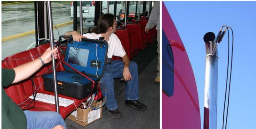
**Figure 3-1. PEMS (left shows system size, right shows tailpipe probe installed in passenger vehicle)**
