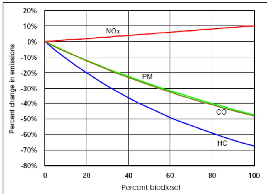
**Figure 1-1. Average emission impacts of biodiesels for heavy-duty vehicle engines (USEPA 2002)**
