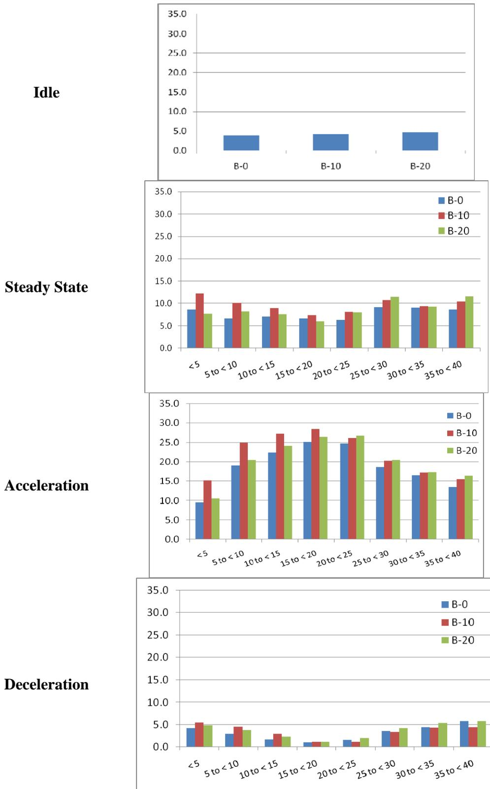
Figure 3-36. CO<sub>2</sub> emissions (g/s) for Bus 997 by mode and speed (mph)
