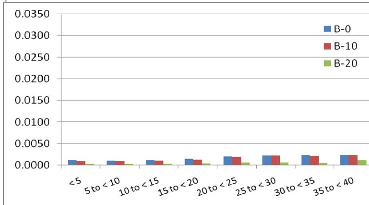
**Figure 3-12. HC emissions (g/s) for Bus 973 by mode and speed (mph)**
