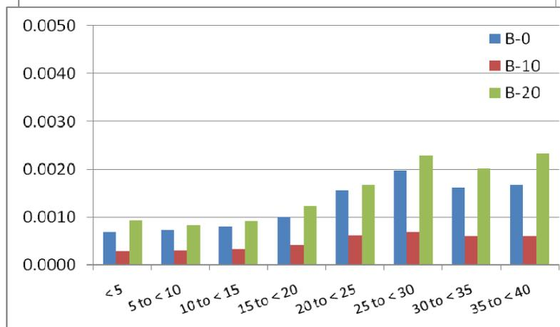
**Figure 3-23. CO emissions (g/s) for Bus 971 by mode and speed (mph)**
