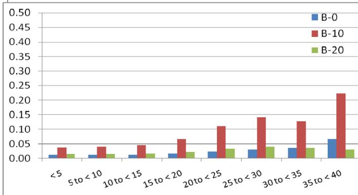
**Figure 3-17. PM emissions (mg/s) for Bus 973 by mode and speed (mph)**
