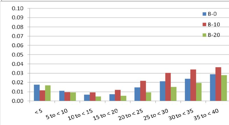
**Figure 3-19. NO<sub>x</sub> emissions (g/s) for Bus 971 by mode and speed (mph)**
