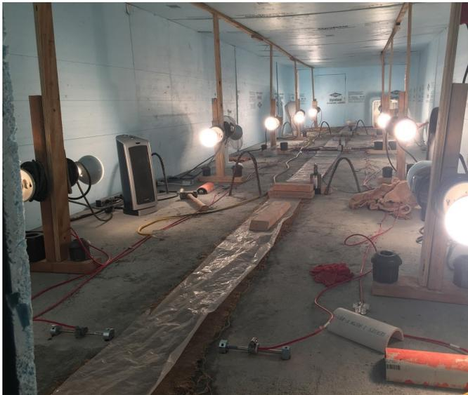
*Temporary temperature isolation room on top of the specimen allowed for the application of heat that would simulate normal thermal radiation consisting of heating of the top surface (Note the joint concrete down the center was covered with burlap, with plastic over that, while the material cured)*
