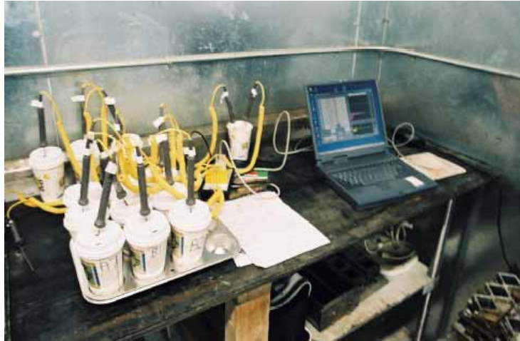
Figure C2. Coffee cup test setup (Gary Knight, Holcim, 10/1/2004 TWP meeting)
