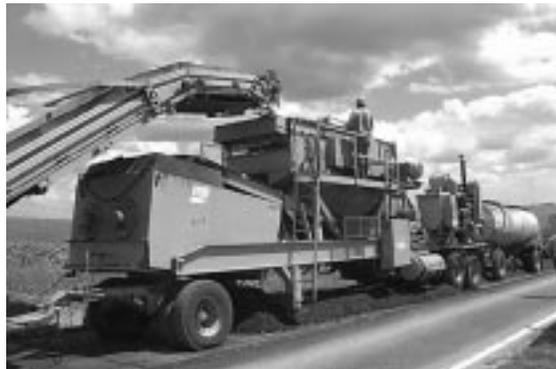
Koss Construction's sizing and rejuvenating portion of the old in-place asphalt recycling train. Photos courtesy of Bryan R. Cawley, ISU research assistant.
