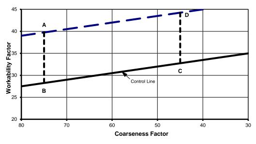
Point A – CF = 75; WF = 40; Point B – CF = 75; WF = 28 Point C – CF = 45; WF = 32; Point D – CF = 45; WF = 44
