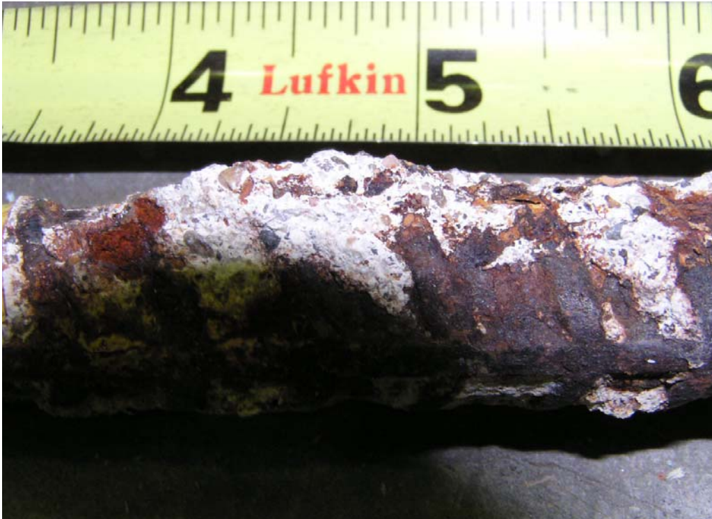
Figure 6.4. Corded uncoated reinforcing bar
