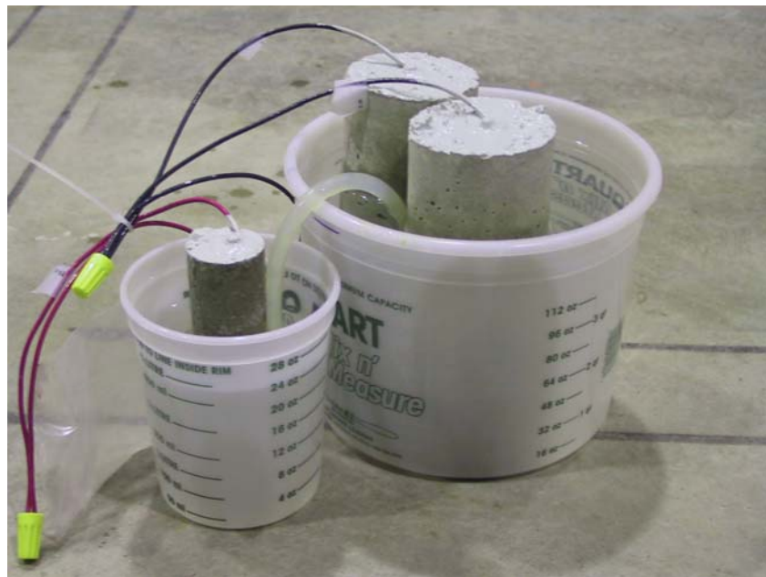
(b) Typical as-constructed Rapid Macrocell ACT
