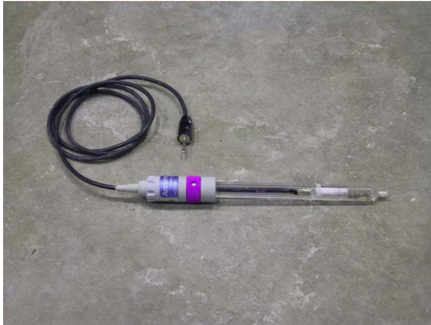
(a) Saturated calomel reference electrode
