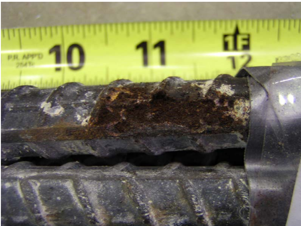
Figure 6.5. Corded MMFX reinforcing bar
