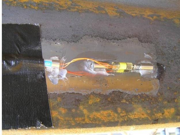
**Figure 5.17. Vibrating-wire strain gauge**
