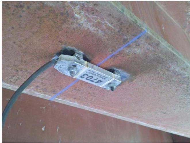
**Figure 5.29. Mounted strain transducer**
