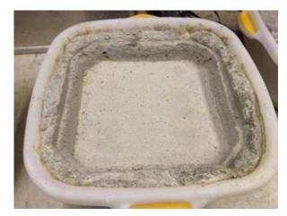
Figure 2. Concrete slab for scaling evaluation
