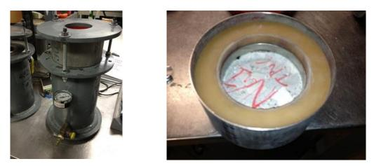
Figure 5. Air permeability apparatus and test specimens sealed tight at the perimeter
