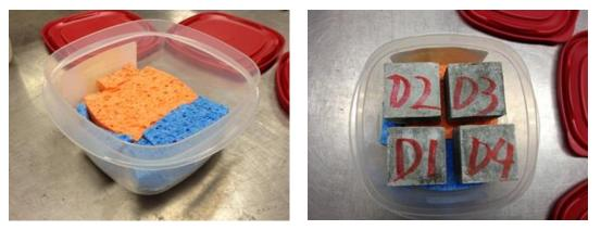
Figure 1. Test cells for cyclic freezing and thawing
