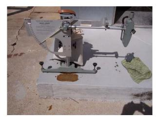
Figure 3. British Pendulum for skid resistance
