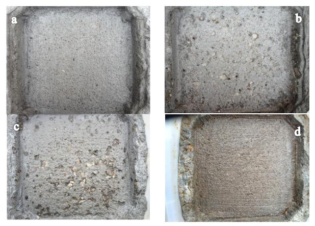
Figure 8. Surface scaling after 50 freezing-thawing cycles: a) plain water, b) 3% sodium chloride, c) 4% calcium chloride, d) Ossian Season One
