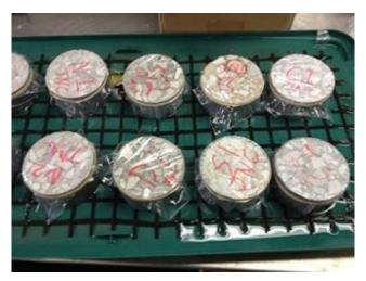
Figure 6. Water absorption specimens
