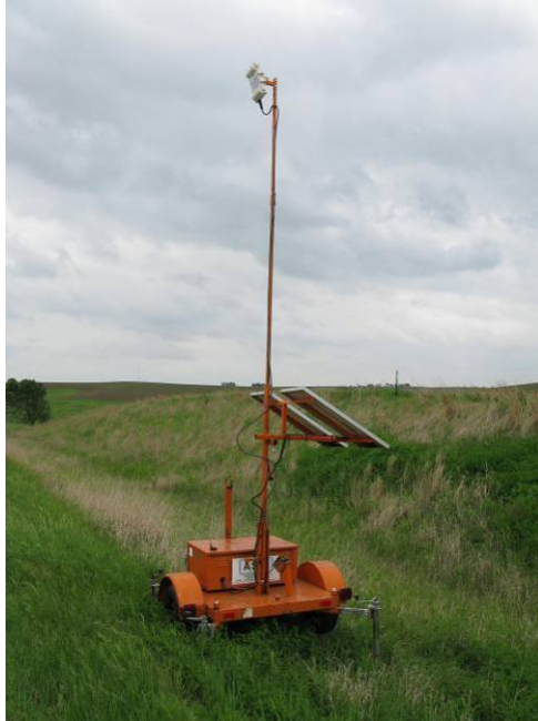
Figure 5. Speed sensor (photo courtesy of Iowa DOT)
