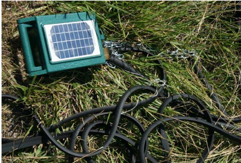
Figure 7. Typical Jamar counter and HD road tubes (photo courtesy of Brad Grefe, CTRE)
