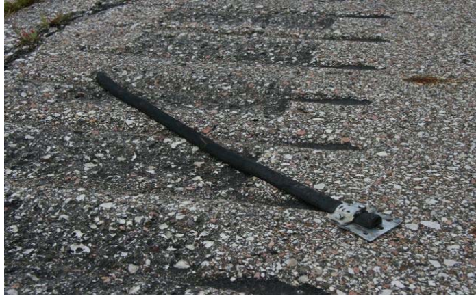
Figure 11. Severed end of road tube (photo by Brad Grefe, CTRE)
