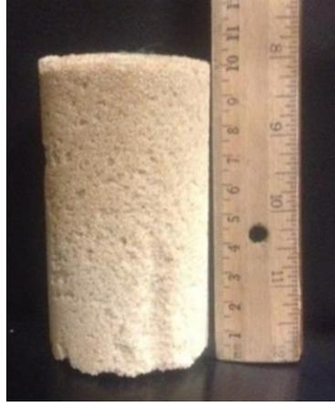
**Figure 6. Cemented sand after MICP treatment**
