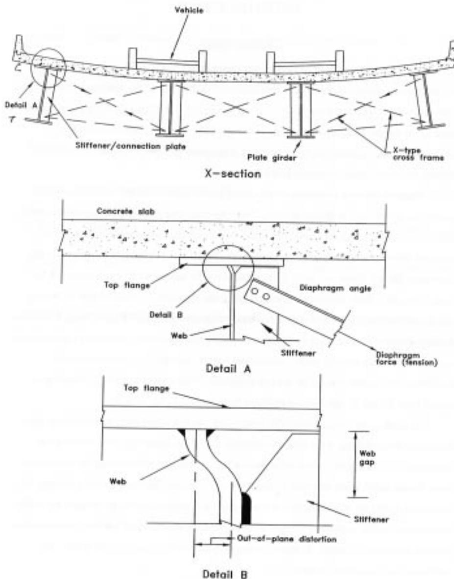
This figure represents out-of-plane girder web distortion in the gap region.
