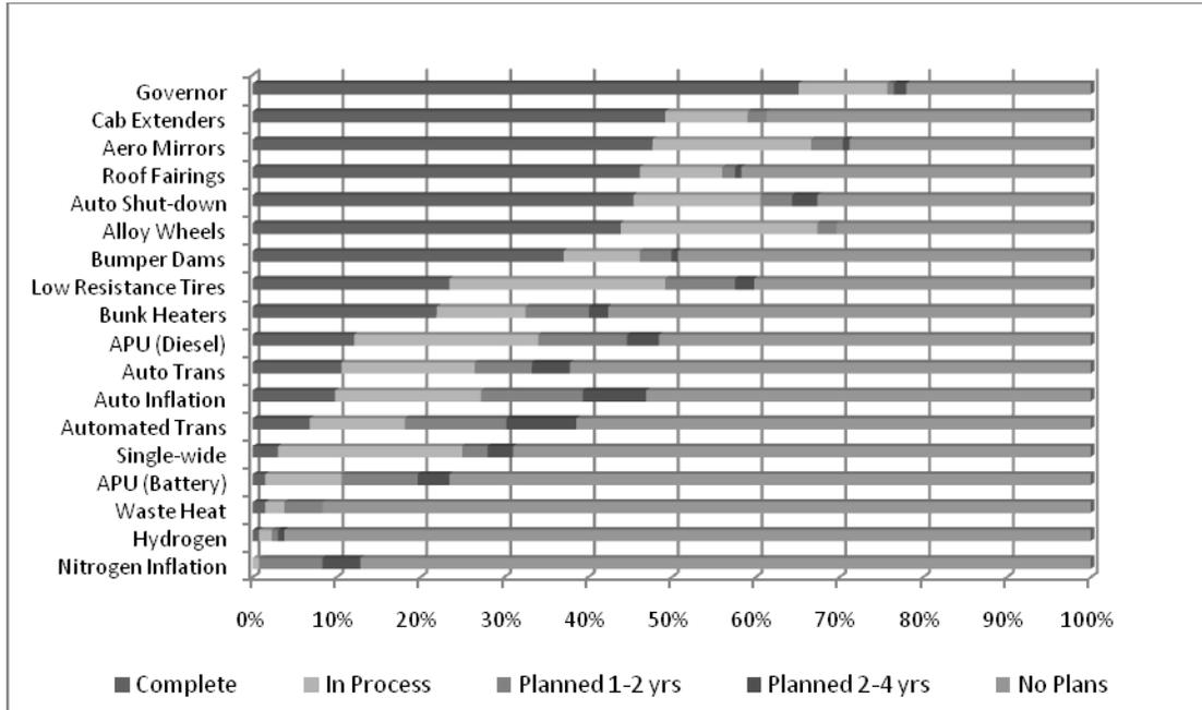
**Figure 6. State of motor unit technology implementation**
