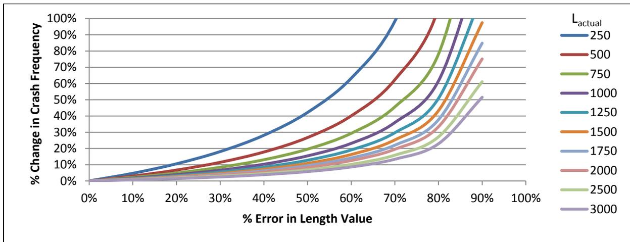
**Figure 10. Safety performance sensitivity to length estimate errors at radius = 1,500 ft**
