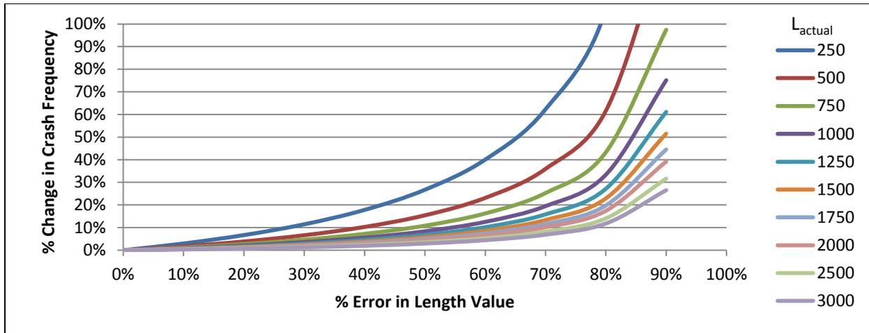
**Figure 11. Safety performance sensitivity to length estimate errors at radius = 3,000 ft**
