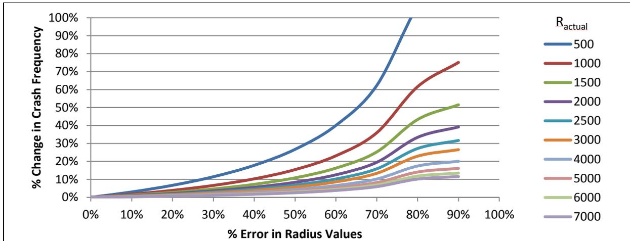
**Figure 8. Safety performance sensitivity to radius estimate errors at length = 3,000 ft**
