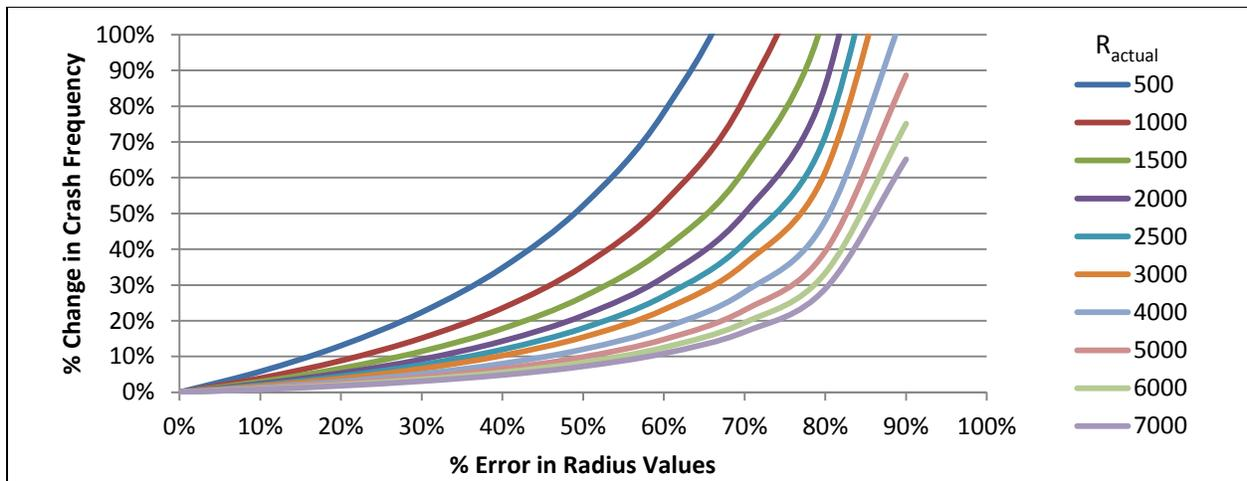
Figure 6. Safety performance sensitivity to radius estimate errors at length = 500 ft
