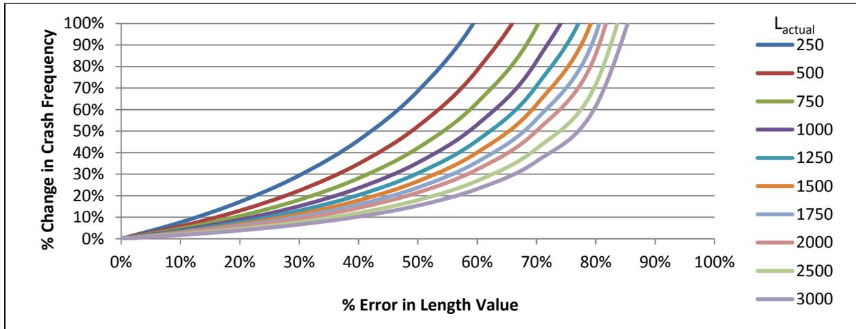
**Figure 9. Safety performance sensitivity to length estimate errors at radius = 500 ft**
