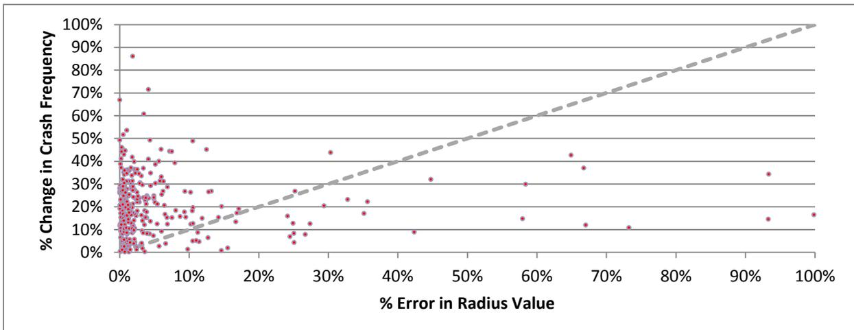
**Figure 13. Crash frequency percent change versus radius estimation error**
