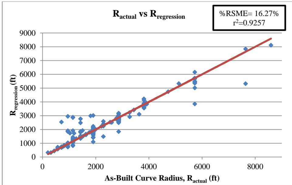
**Figure 4. Actual versus circular regression estimated radius**
