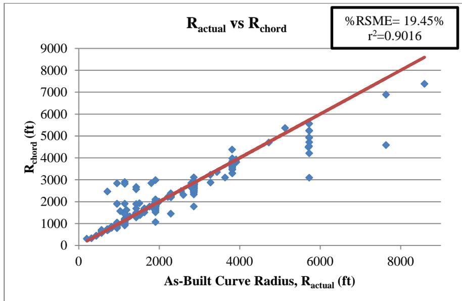
**Figure 5. Actual versus long chord estimated curve radius**
