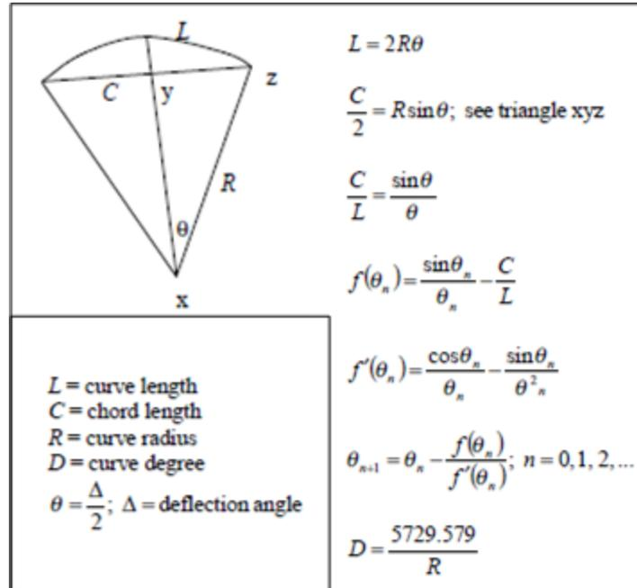
**Figure 2. Newton iteration of curve radius**
