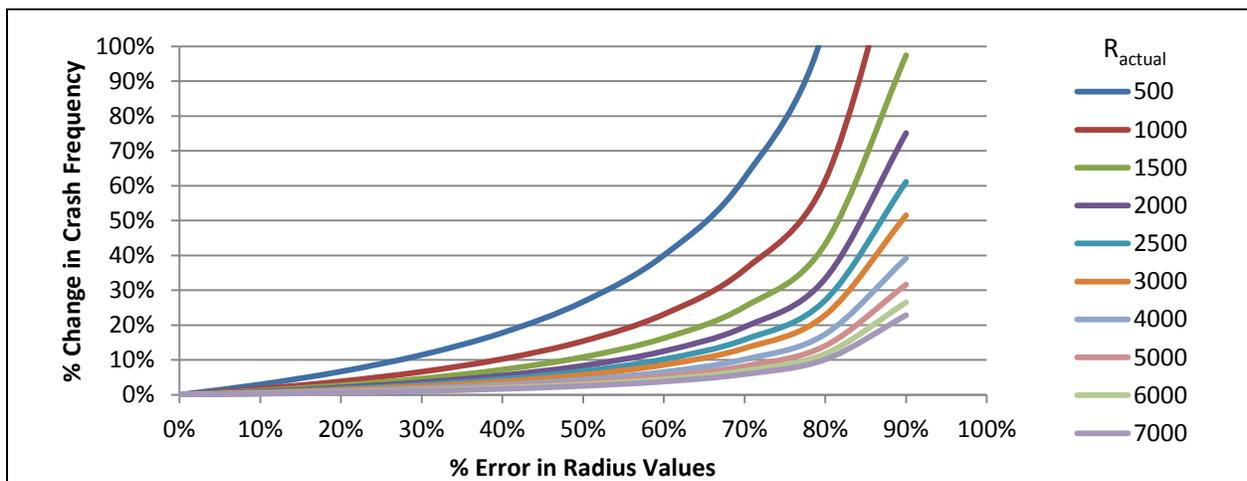
Figure 7. Safety performance sensitivity to radius estimate errors at length = 1,500 ft
