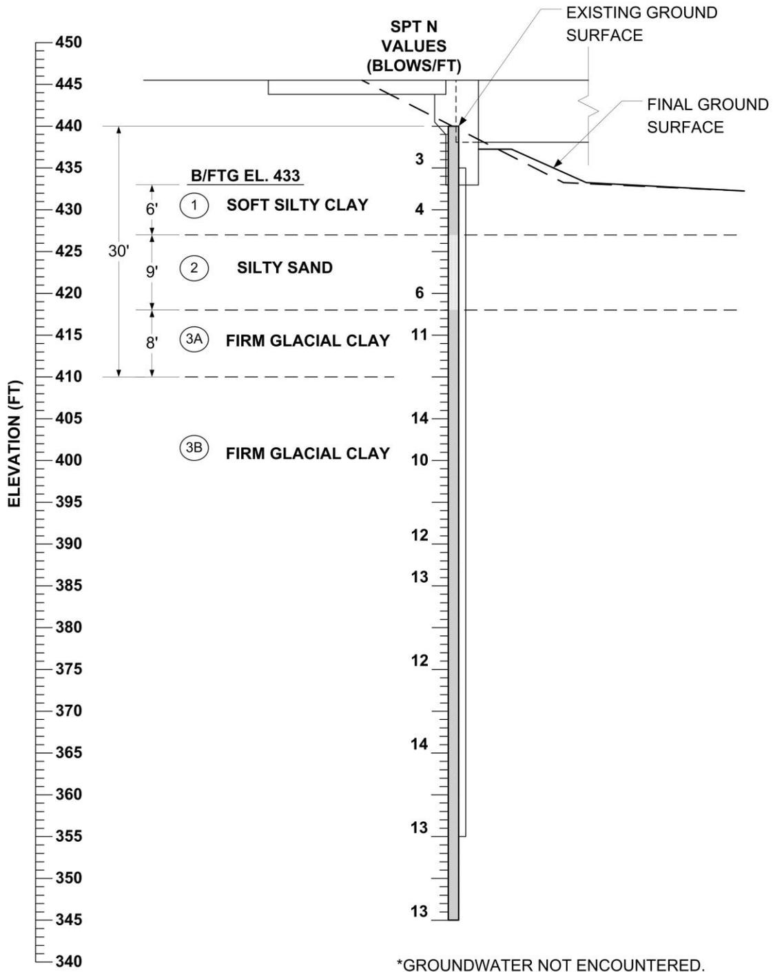
Figure 3.1. Track 1 Example 1: Soil profile
