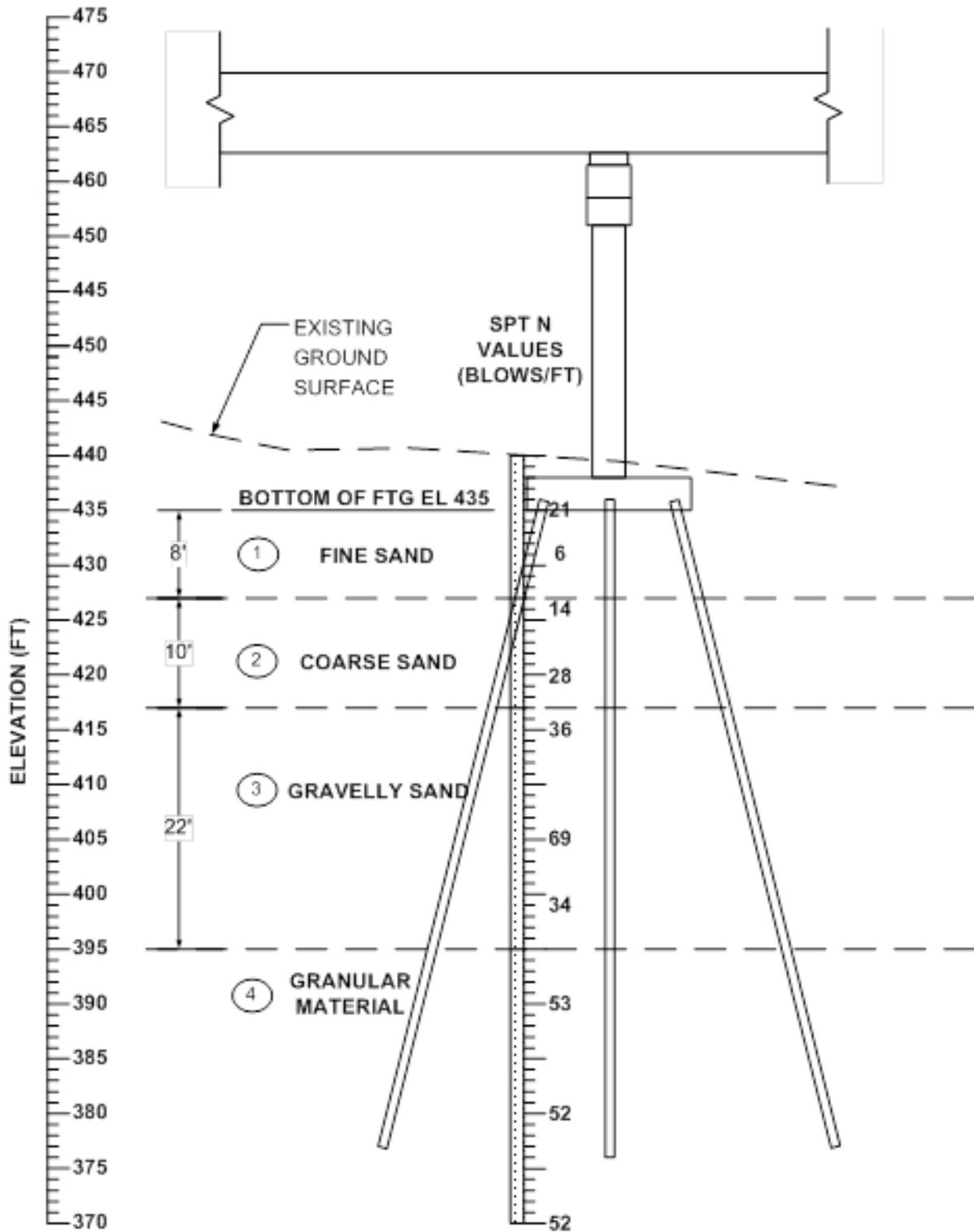
Figure 3.13. Track 1 Example 4: Soil profile
