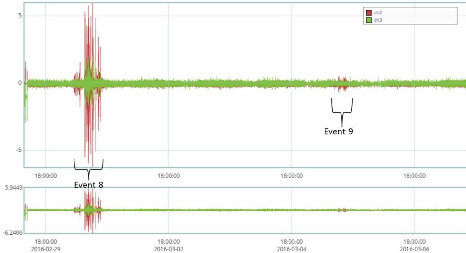
Figure 14. Typical acceleration data from a vertical member showing two “events”
