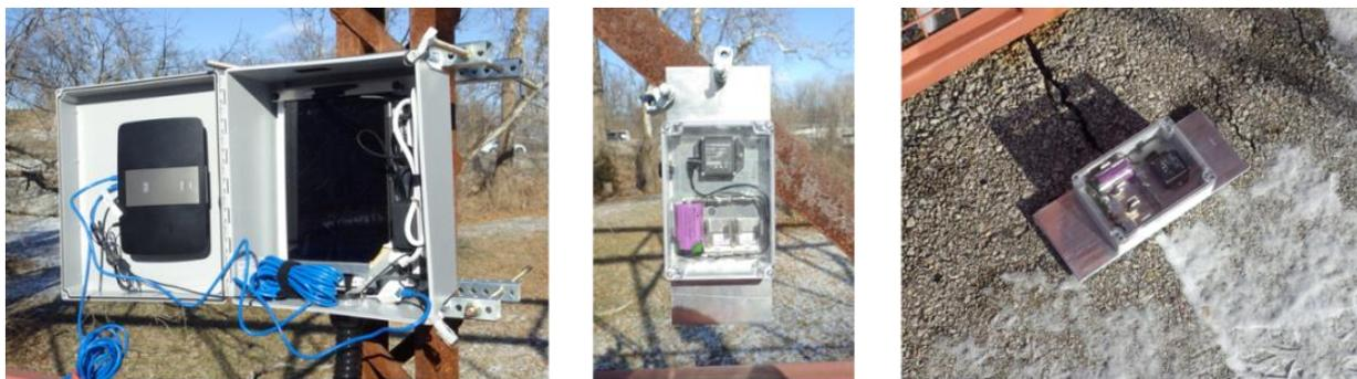
**Figure 8. Attachment of the data acquisition system (left), attachment of sensor to a tension tie (middle), and placement of sensor on the deck (right) during field implementation test**
