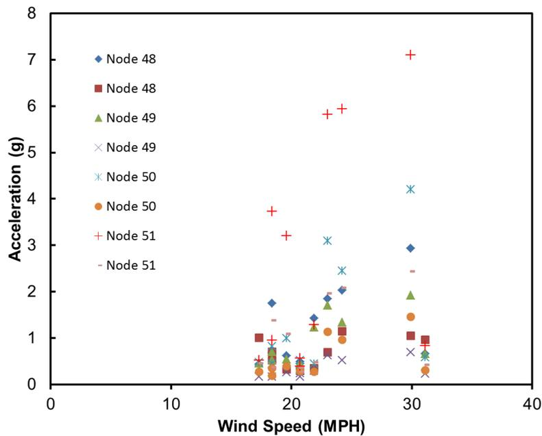
**Figure 16. Correlation between maximum winds and maximum accelerations**
