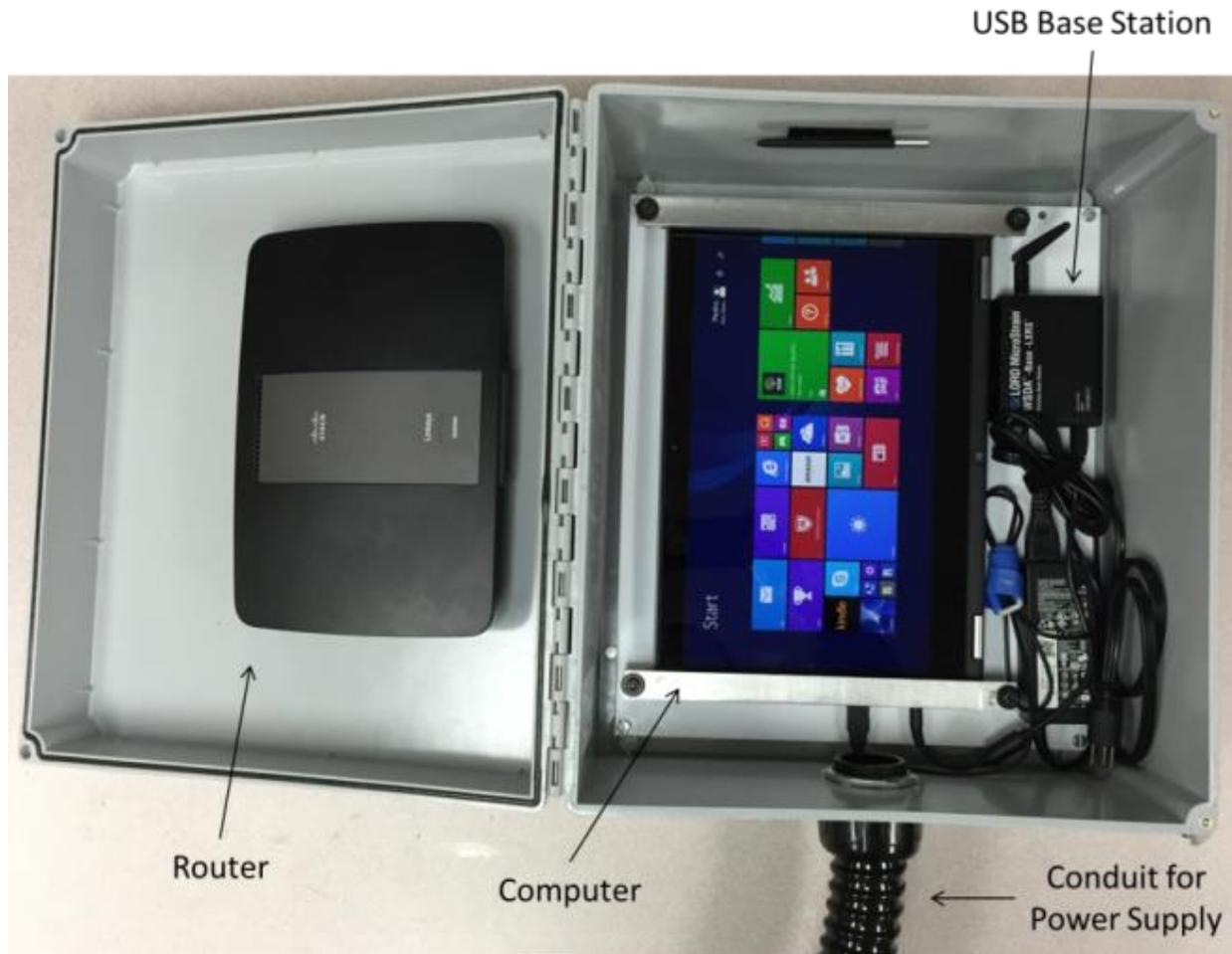
**Figure 3. Data acquisition system integrated with essential components**
