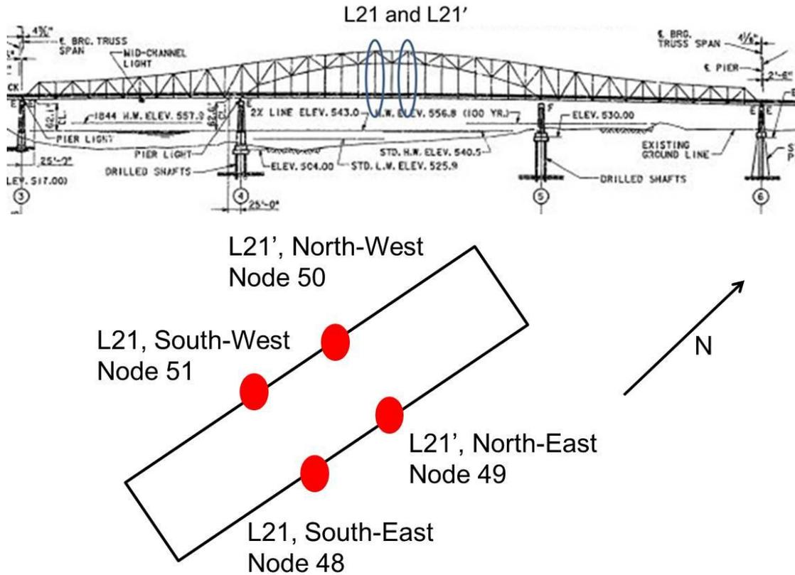
**Figure 12. Location of sensor nodes mounted on verticals L21 and L21'**
